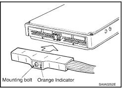
For removal of the lever type connector, pull the lever up to the direction pointed to by the arrow A in the figure, and then remove the connector.
