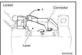
For installation of the lever type connector, pull down the lever to the direction pointed by the arrow B in the figure, and then push the connector until a clicking noise is heard.
