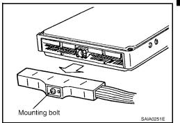
Before installing a connector, make sure the terminal is not bent or damaged, and then correctly connect it. When installing a connector by tightening bolts, fix it by tightening the mounting bolt until the painted projection of the connector becomes even with the surface.
