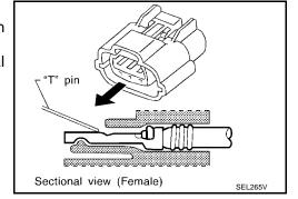
Some connectors do not have a notch above each terminal. To probe each terminal, remove the connector retainer to make contact space for probing.
