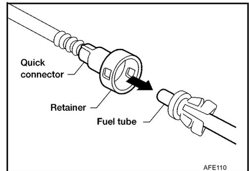
● Insert tube into the center of the connector until you hear a click. After connecting quick connectors, make sure the connection is fully seated and locked in place as follows:
