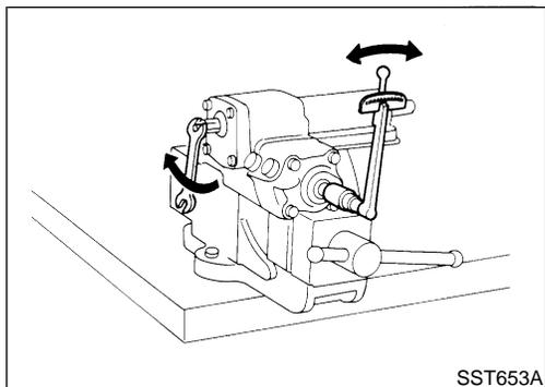
d. Measure turning torque at straight-ahead position.
