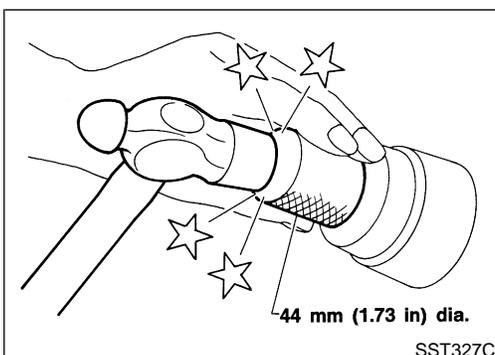
9. Install new oil seal into gear housing with suitable tool.
