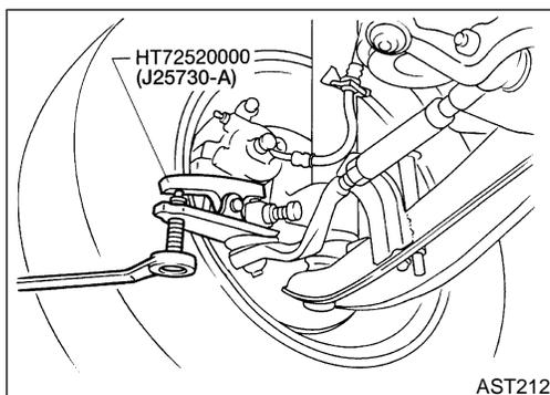
Remove tie-rod from knuckle arm with Tool.
