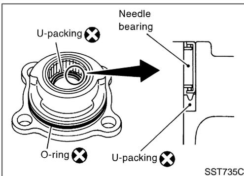
6. Install new O-ring into sector shaft cover.
