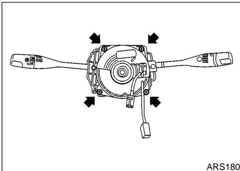
8. Remove the four spiral cable retaining screws. Remove the spiral cable.
