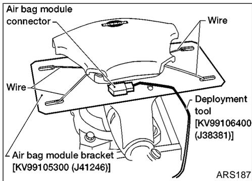
3. Connect deployment tool [SST: KV99106400 (J38381)] to driver air bag module connector.
