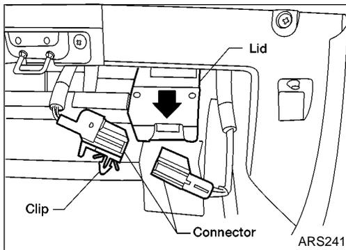
3. Connect passenger air bag module connector to air bag harness connector.
