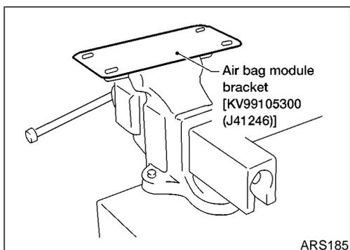
2. Firmly secure air bag module bracket [SST: KV99105300 (J41246)] in a vise.
