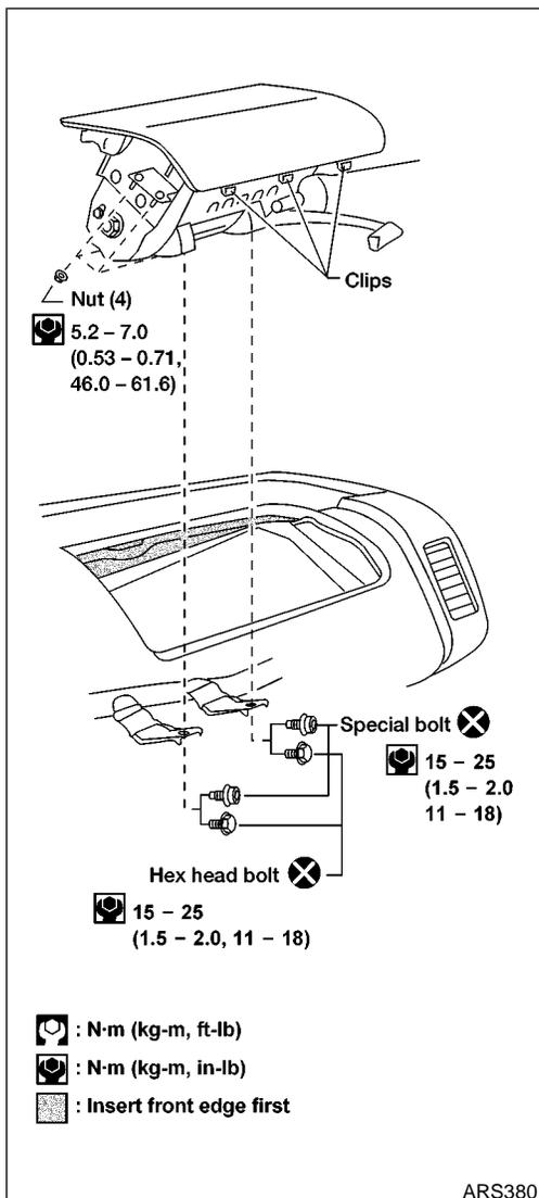
6. Remove two hex head bolts or if required use TAMPER RESISTANT TORX (Size T50) to remove the two special bolts.
