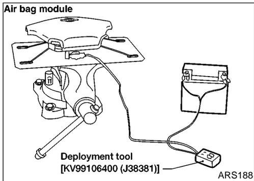
4. Connect red clip of deployment tool [SST: KV99106400 (J38381)] to battery positive terminal and black clip to negative terminal.
