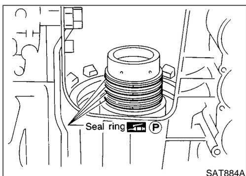
9. Install low one-way clutch inner race seal ring.
