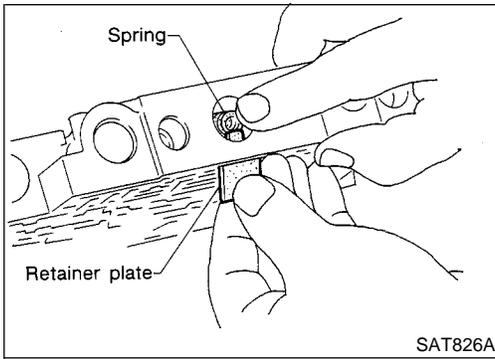
b. Remove retainer plates while holding spring.
