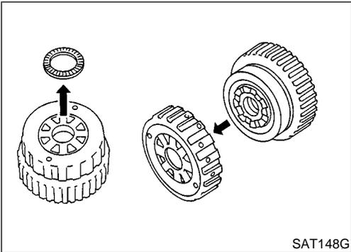
e. Remove needle bearing from overrun clutch hub.
