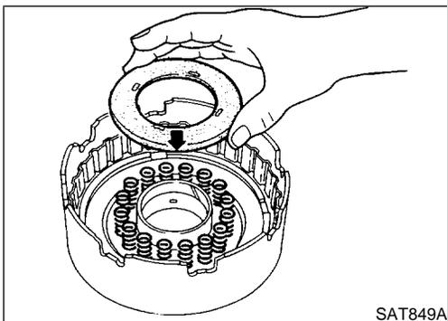
3. Install return springs and spring retainer.
