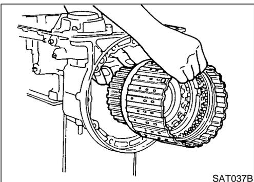
h. Remove forward clutch assembly from transmission case.
