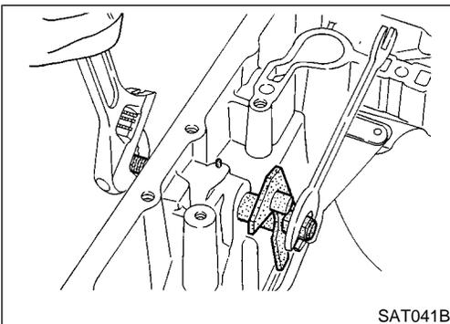
22. Remove manual shaft components, if necessary.
