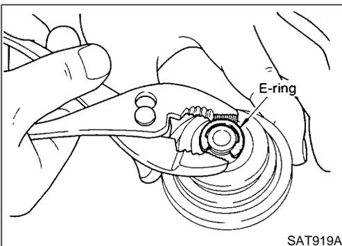
3. Install E-ring onto servo cushion spring retainer.
