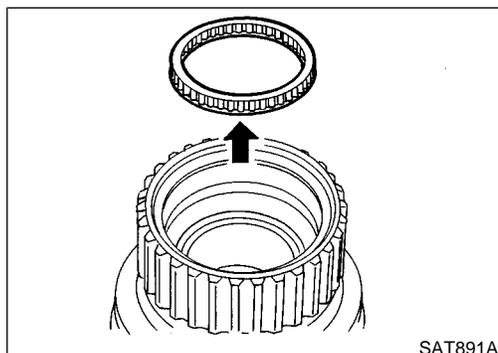
5. Remove needle bearing from forward clutch drum.
