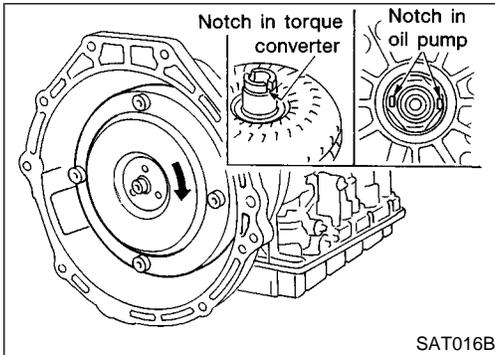
b. Install torque converter while aligning notches and oil pump.
