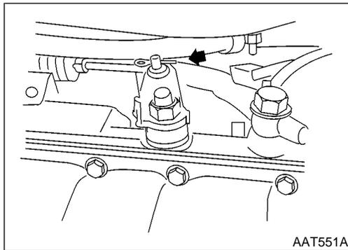
2. If NG, check again with manual control linkage disconnected from manual shaft of A/T assembly. Refer to step 1.
