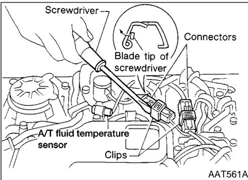
8. Remove torque converter clutch solenoid valve and A/T fluid temperature sensor connectors.
