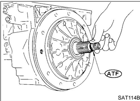
5. Install O-ring on input shaft.
