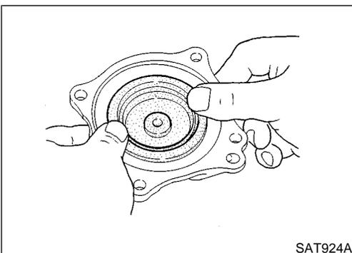
9. Install OD band servo piston onto servo piston retainer by pushing it inward.
