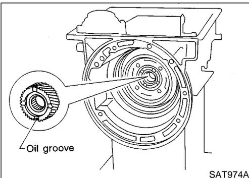
7. Install front side clutch and gear components.
