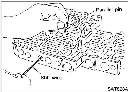
● 4-2 sequence valve and relay valve are located far back in upper body. If they are hard to remove, carefully push them out using stiff wire.
