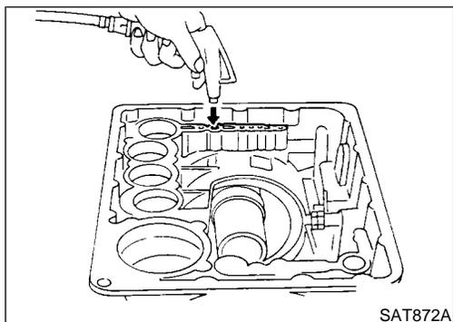
7. Check operation of low and reverse brake clutch piston. Refer to "DISASSEMBLY", AT-306.
