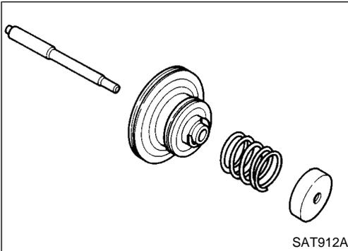
5. Install servo piston spring retainer, return spring C and piston stem onto band servo piston.
