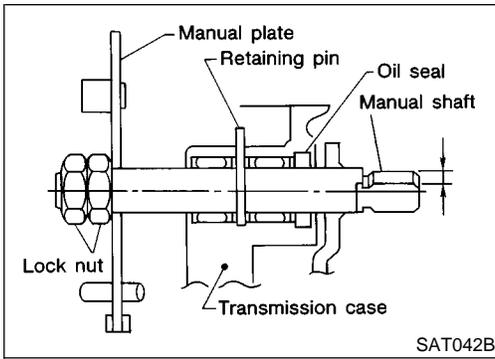
b. Remove retaining pin from transmission case.
