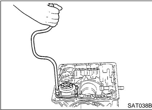
21. Remove band servo and accumulator components.
