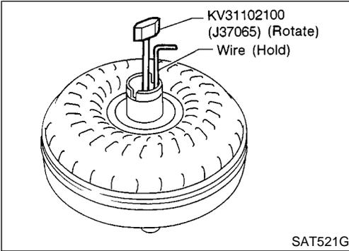
3. Check torque converter one-way clutch.
