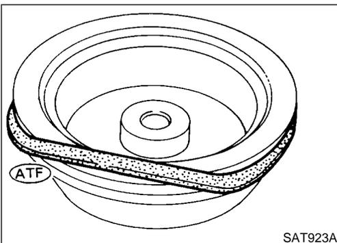
8. Install D-ring on OD band servo piston.
