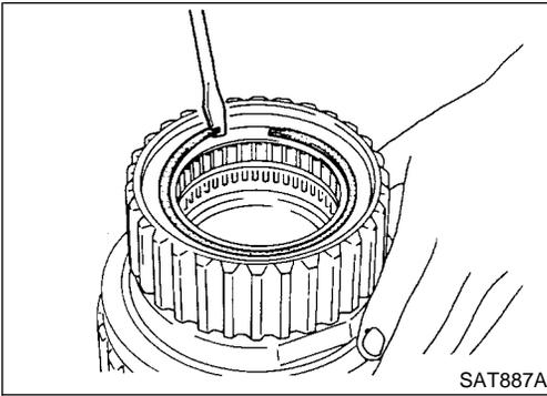
4. Install side plate onto forward clutch drum.
