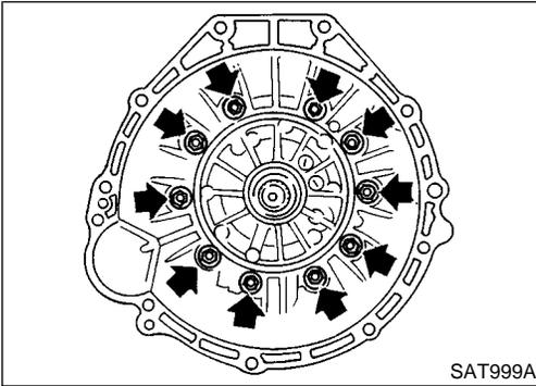
12. Remove converter housing from transmission case.
