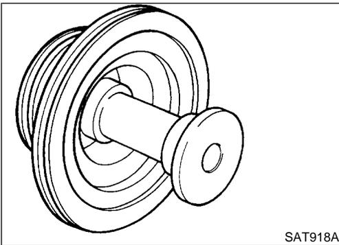
2. Install servo cushion spring retainer onto band servo piston.
