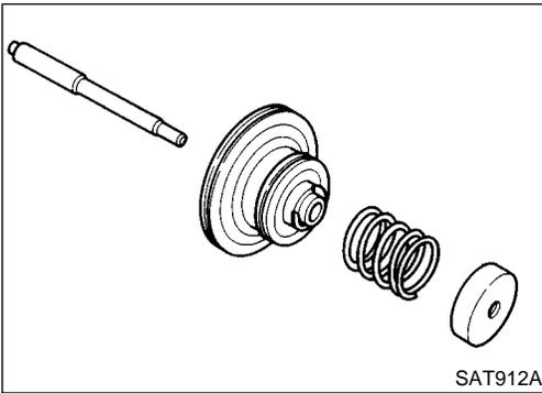
6. Remove servo piston spring retainer, return spring C and piston stem from band servo piston.
