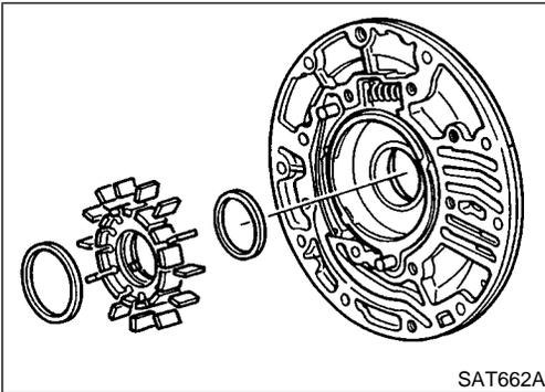
3. Install rotor, vanes and vane rings.
