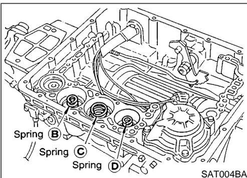
9. Install control valve assembly.
