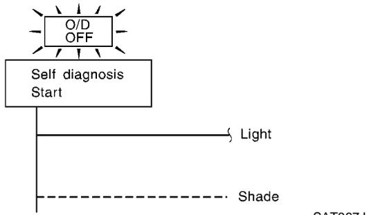
PNP switch, overdrive control switch or throttle position switch circuit is disconnected or TCM is damaged.
