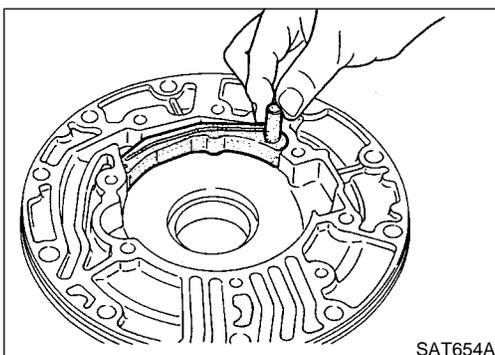
2. Install cam ring in oil pump housing by the following
