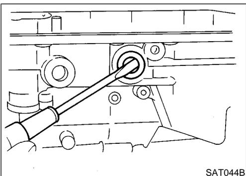
f. Remove oil seal from transmission case.
