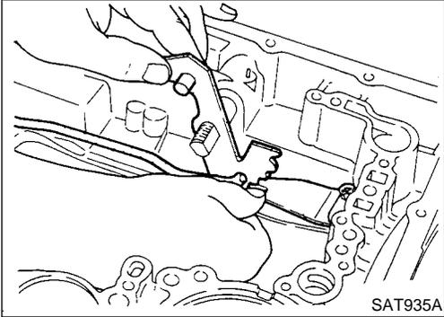
c. While pushing detent spring down, remove manual plate and parking rod from transmission case.
