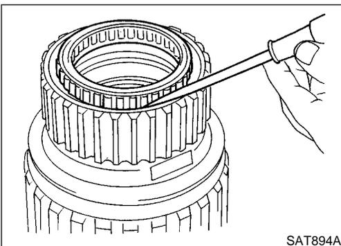
3. Install low one-way clutch onto forward clutch drum by pushing the roller in evenly.
