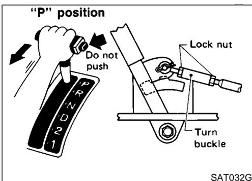
3. Tighten turn buckle until aligns with inner cable, pulling selector lever toward R position side without pushing button.
