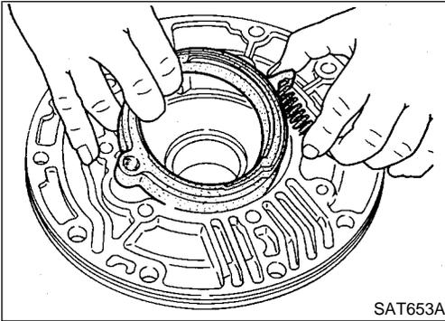
5. Remove cam ring and cam ring spring from oil pump housing.
