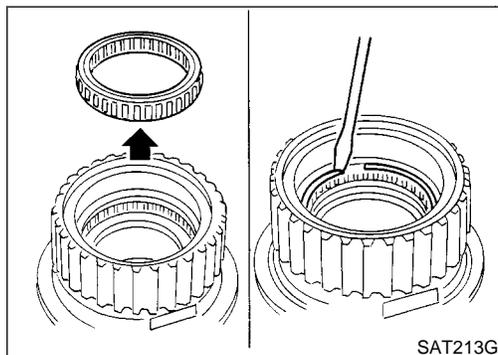
3. Remove low one-way clutch from forward clutch drum.
