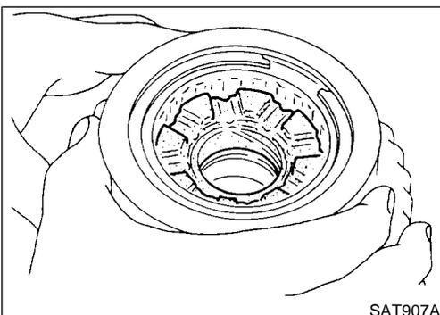
7. Position forward clutch hub in rear internal gear.
