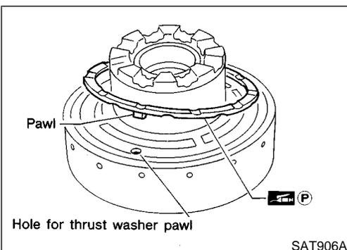
6. Install thrust washer onto rear internal gear.
