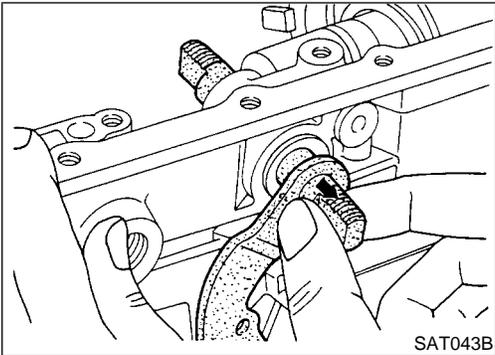
d. Remove manual shaft from transmission case.
