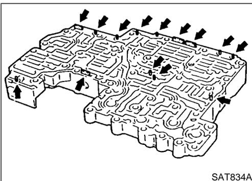
2. Install parallel pins and retainer plates.
