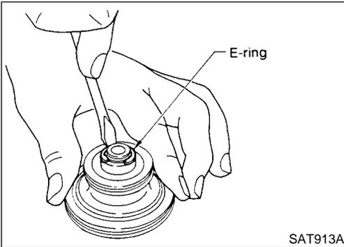
7. Remove E-ring from band servo piston.
