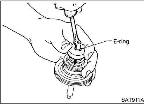
5. Place piston stem end on a wooden block. While pushing servo piston spring retainer down, remove E-ring.
