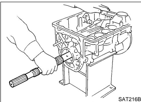
5. Install output shaft and parking gear.
