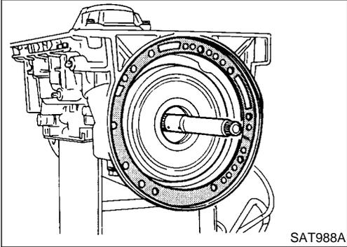
15. Remove input shaft and oil pump gasket.
