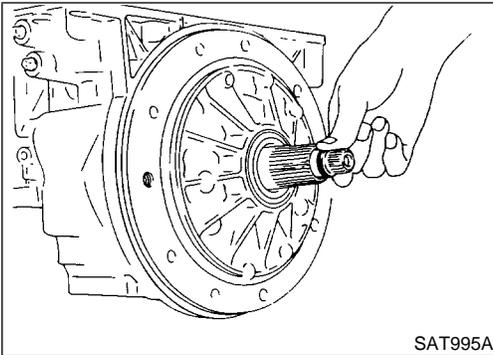
13. Remove O-ring from input shaft.
