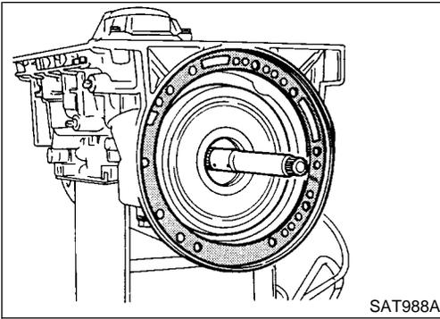
2. Install input shaft on transmission case.
