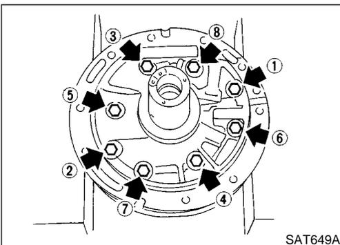
4. Install oil pump housing and oil pump cover.
