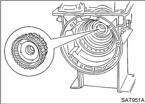
d. Remove rear internal gear, forward clutch hub and overrun clutch hub as a set from transmission case.
