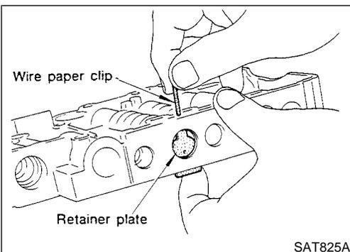
2. Remove valves at retainer plates.
