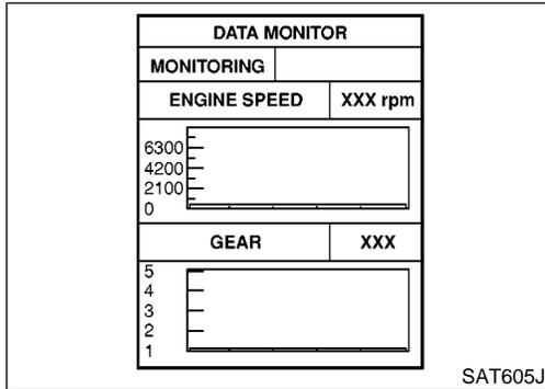
11. After finishing cruise test part 1, touch "STOP".
