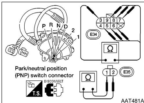
4. If NG on step 2, remove PNP switch from A/T and check continuity of PNP switch terminals. Refer to step 1.
