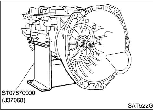
6. Place transmission into Tool with the control valve facing up.
