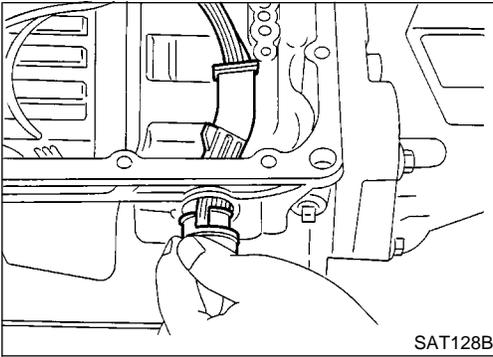
11. Remove terminal cord assembly from transmission case while pushing on stopper.
