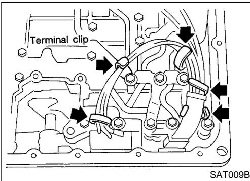
10. Remove control valve assembly.
