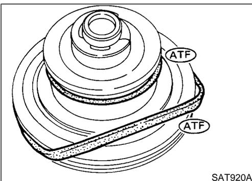
4. Install D-rings onto band servo piston.
