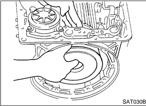
17. Remove front side clutch and gear components.
