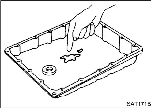
7. Check foreign materials in oil pan to help determine cause of malfunction. If the fluid is very dark, smells burned, or contains foreign particles, the frictional material (clutches, band) may need replacement. A tacky film that will not wipe clean indicates varnish build up. Varnish can cause valves, servo, and clutches to stick and may inhibit pump pressure.
