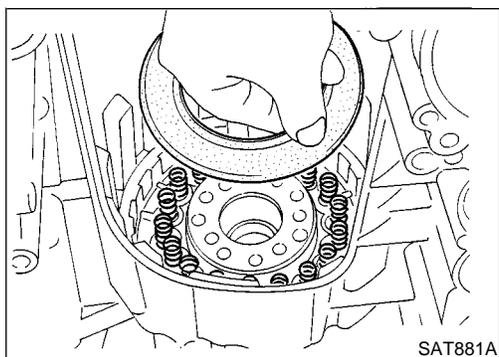
4. Install return springs, spring retainer and low one-way clutch inner race onto transmission case.
