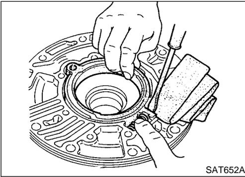
4. While holding cam ring and spring lift out cam ring spring.
