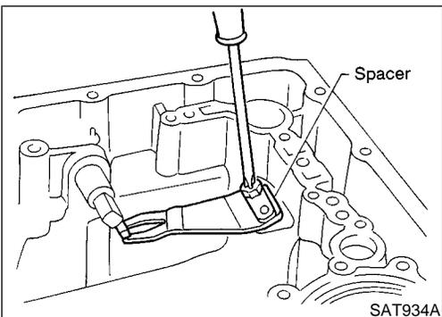
e. Remove spacer and detent spring from transmission case.
