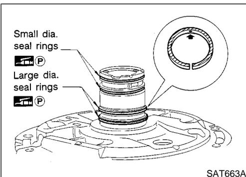
5. Install new seal rings carefully after packing ring grooves with petroleum jelly. Press rings down into jelly to a close fit.
