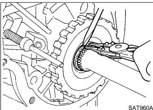
19. Remove output shaft and parking gear.
