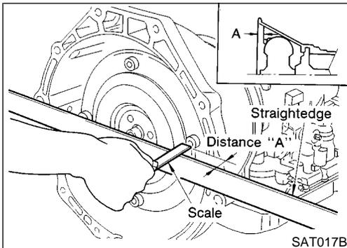
c. Measure distance A to check that torque converter is in proper position.
