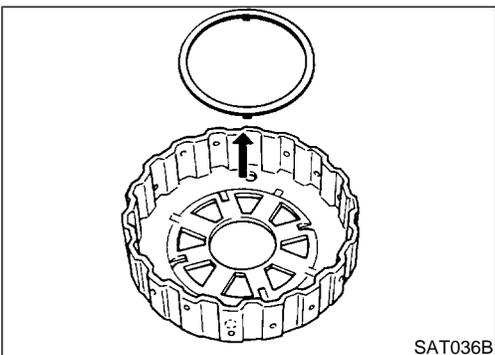
g. Remove thrust washer from overrun clutch hub.
