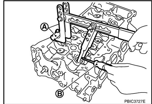
5. Remove valve spring retainer, valve spring and valve spring seat.
