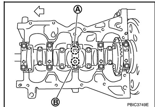
7. Tighten main bearing cap bolts in numerical order shown with the following steps.
