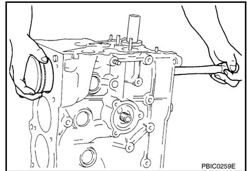
13. Remove connecting rod bearings.
