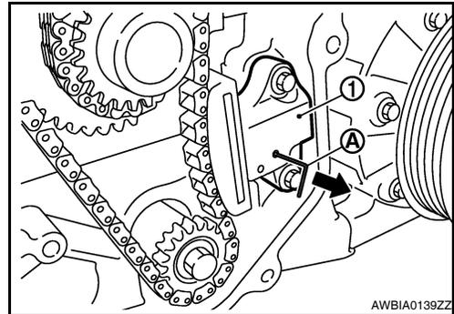
6. Align the matching marks of each sprocket with the matching marks of timing chain.
