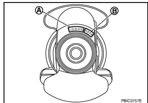
3. Read the symbol at the cross point of selected row and column in the "Main Bearing Selection Table".
