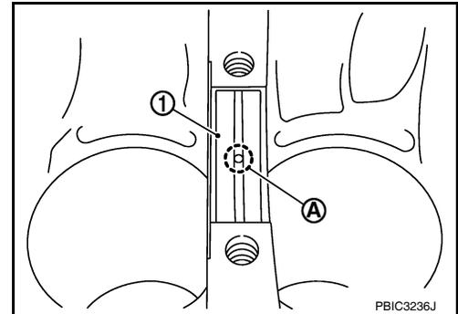
6. Install signal plate to crankshaft if removed.
