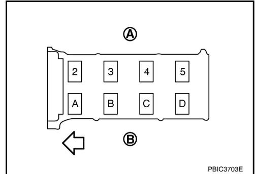
13. Tighten bolts of camshaft brackets in the following steps, in numerical order as shown.
