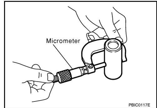
Piston to Piston Pin Oil Clearance
