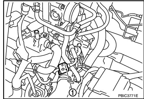
4. With the sleeve side of quick connector release facing quick connector, install quick connector release onto fuel tube.
