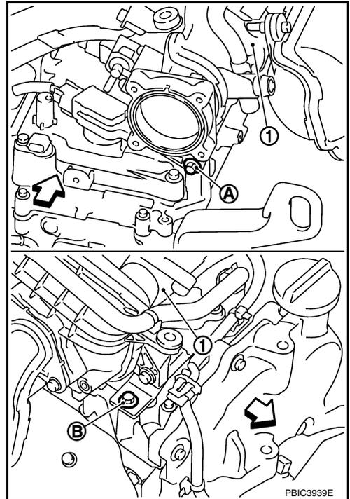
6. Loosen remaining intake manifold bolts in the reverse order as shown.
