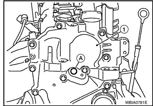
5. Install engine mounting bracket (RH), engine mounting insulator, and torque rod (RH) under the Step 4 condition. (With intake valve timing control solenoid valve removed, and a shop cloth inserted into the oil hole.) Refer to [EM-195. "Component"](#).
