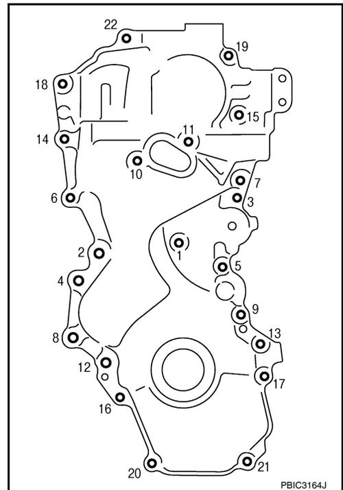
13. Cut liquid gasket by prying the position (■) shown, and then remove the front cover.
