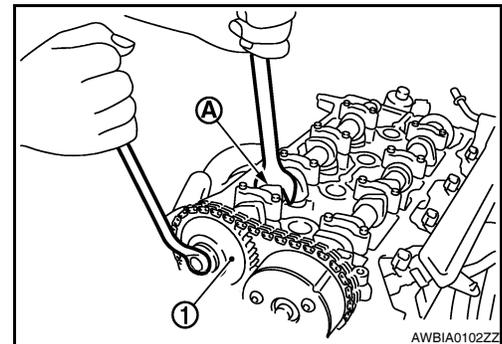
12. Turn the camshaft sprocket (INT) to the most advanced position.
