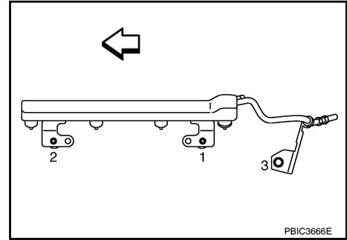
7. Remove the fuel injector (3) from the fuel tube (1) with the following procedure.
