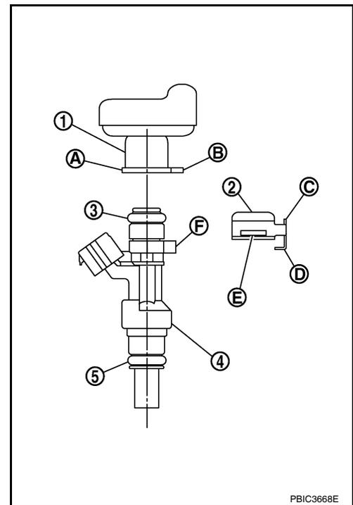
3. Install fuel tube and injector assembly onto cylinder head.
