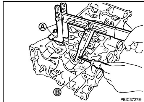
4. Remove valve spring retainer and valve spring.
