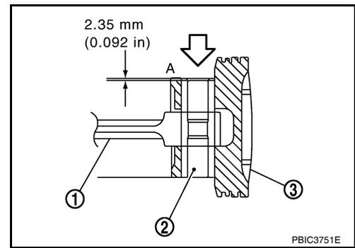
9. Using a suitable tool, install piston rings.
