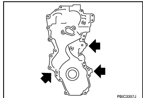
14. Remove front oil seal from front cover.
