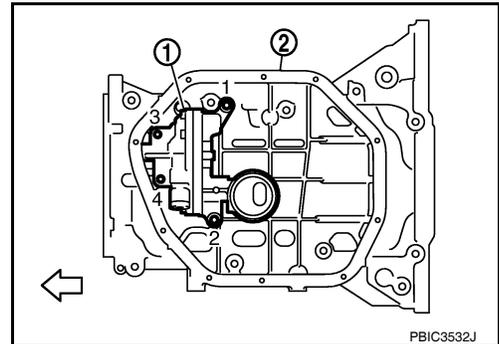
8. Use a scraper (A) to remove old liquid gasket from mating surfaces of oil pan (lower).
