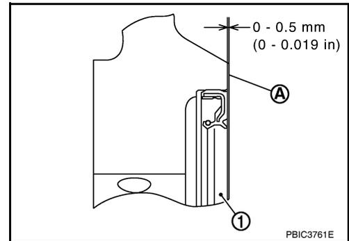
3. After press-fitting rear oil seal, completely wipe off any liquid gasket protruding to rear end surface side.
