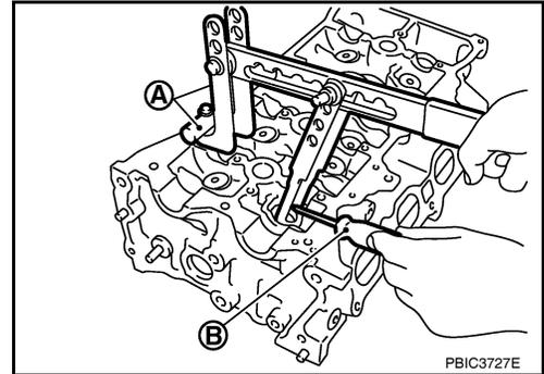
5. Remove valve spring retainer, valve spring and valve spring seat. Refer to [EM-82. "Disassembly and Assembly"](#).
