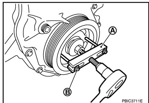
9. Remove front cover with the following procedure:
