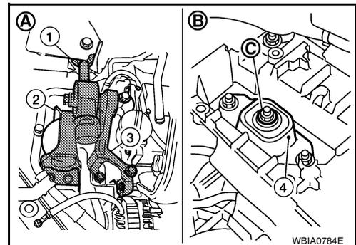
31. Remove the engine and the transaxle assembly from the vehicle downward by carefully operating supporting tools.
