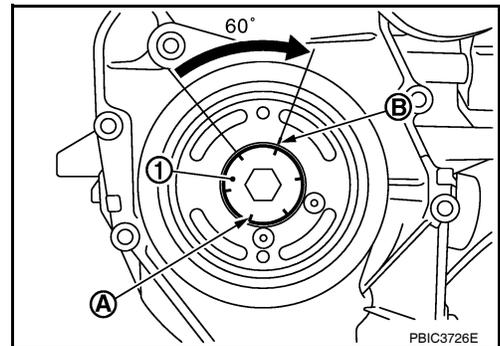
10. Make sure that crankshaft turns smoothly by rotating by hand clockwise.
