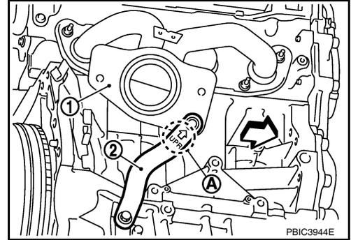
4. Install the air fuel ratio sensor 1, using Tool (A).
