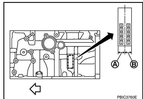
2. Apply main journal diameter grade stamped on crankshaft front side to column in the "Main Bearing Selection Table".
