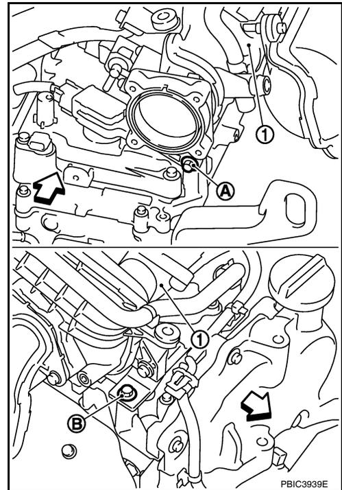
4. Install electric throttle control actuator.
