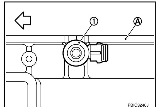
28. Install crankshaft position sensor (POS) and crankshaft position sensor (POS) cover.
