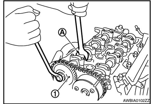
12. Install camshaft brackets (No. 2 to 5) aligning the identification marks on upper surface as shown.
