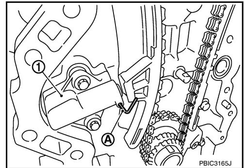
9. Check matching mark position of timing chain and each sprocket again.
