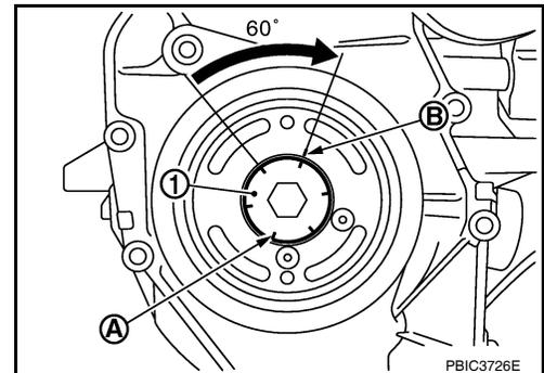
24. Make sure that crankshaft turns smoothly by rotating by hand clockwise.
