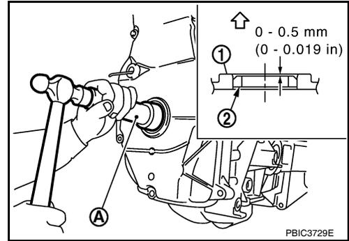
12. Install new O-ring to cylinder block.
