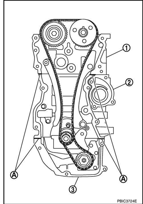
b. Apply a continuous bead of liquid gasket with Tool to front cover as shown.
