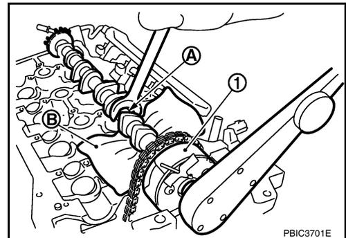
9. Return the camshaft (INT) to the cylinder head carefully.
