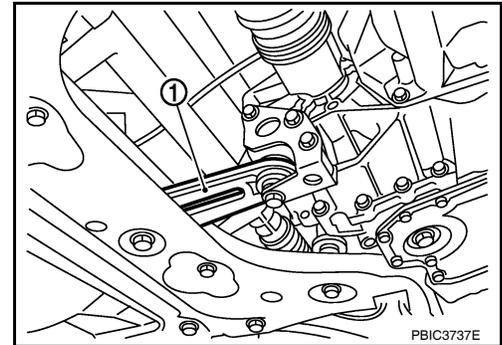
6. Remove A/T cooler hoses from transmission (if equipped).
