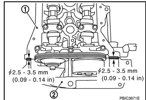
2. Install rocker cover to the cylinder head.
