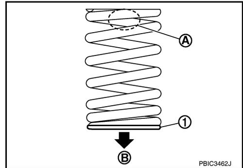
6. Install valve spring retainer.
