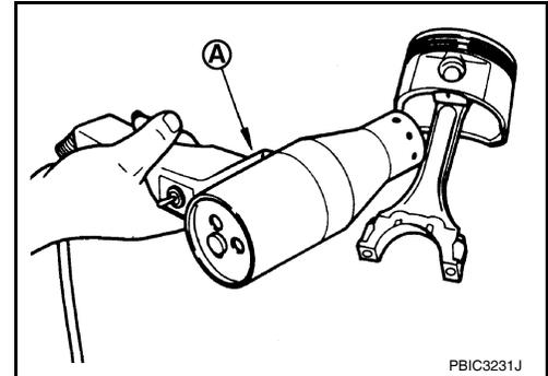
18. Push out piston pin using a suitable tool of an outer diameter approximately 18 mm (0.71 in).
