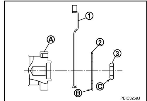
27. Install knock sensor (1) with connector facing toward the rear of engine.
