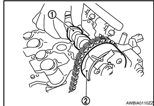
7. Put a thick shop cloth (B) to the lower surface, and then set the tools to the bolt camshaft (INT) (1).
