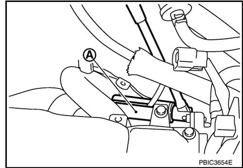
6. Remove exhaust manifold side bolt of exhaust manifold stay.
