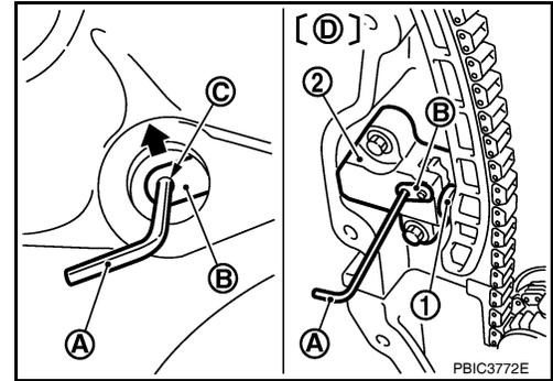
19. Return the camshaft sprocket (INT) in the most retarded position with the following procedure.
