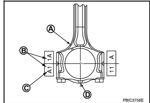
2. Apply crankshaft pin journal diameter grade stamped (B) on crankshaft front side to the column in the "Connecting Rod Bearing Selection Table".
