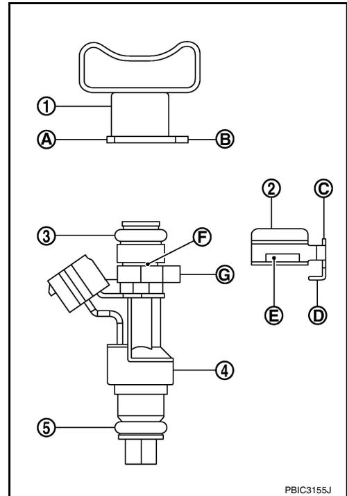
3. Set fuel tube and fuel injector assembly at its position for installation on cylinder head.
