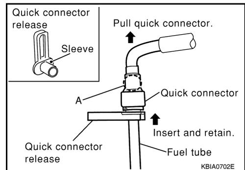
6. Draw and pull out quick connector straight from fuel tube.
