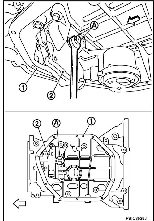
5. Install chain tensioner (for oil pump) (1).
