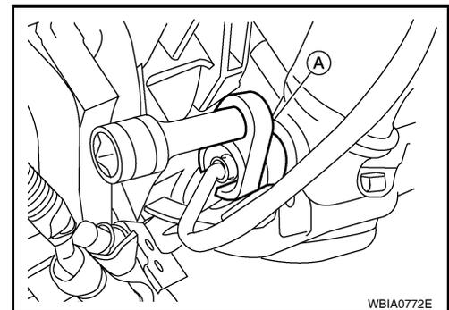
4. Remove exhaust manifold side bolt of exhaust manifold stay.
