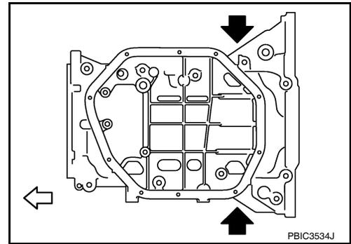
11. After removing the bolts, separate the mating surface and remove the sealant using Tool.
