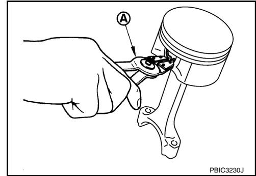
17. Heat piston to 60° to 70°C (140° to 158°F) using a suitable tool (A).
