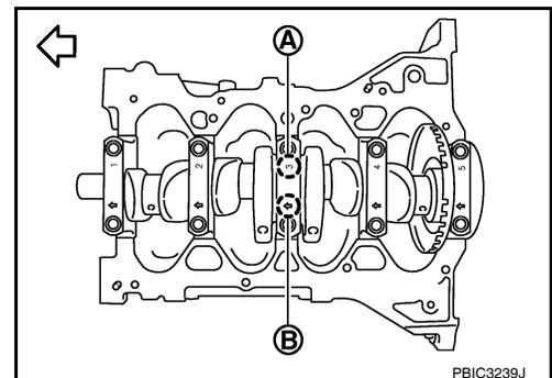
14. Apply new engine oil to threads and seat surfaces of bolts.
