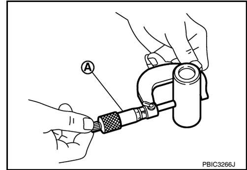
Connecting Rod Bushing Oil Clearance
