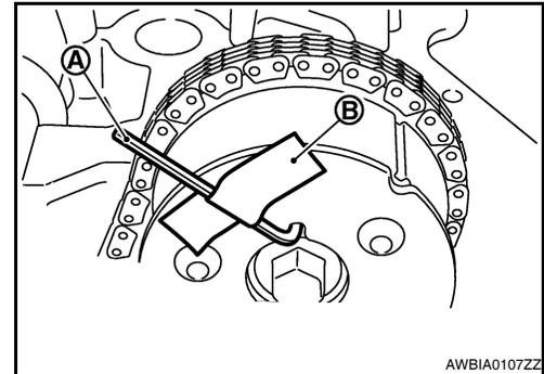
b. Turn the crankshaft slowly clockwise and return the camshaft sprocket (INT) to the most retarded angle position.
