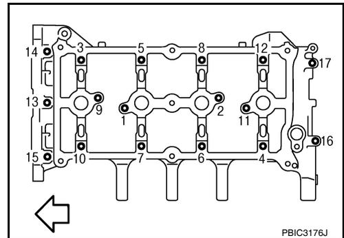
11. Cut liquid gasket by prying the position (■) shown, and then remove the camshaft bracket.
