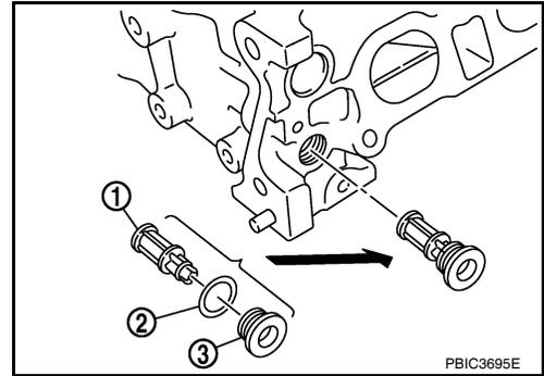
2. Install intake valve timing control solenoid valve.
