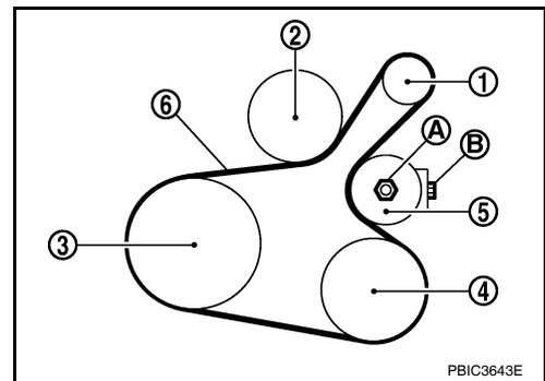
**Idler pulley lock nut : 4.4 N·m (0.45 kg-m, 39 in-lb)**
