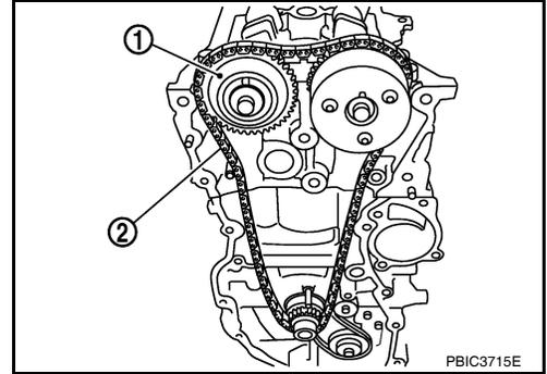
14. Remove the crankshaft sprocket and the oil pump drive related parts with the following procedure.
