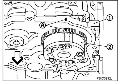
9. Remove camshaft sprockets (INT) (1) and (EXH) (2).
