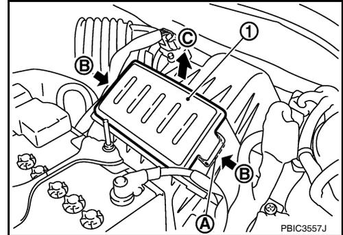
3. Remove the air cleaner filter (1) and holder (2) assembly from the air cleaner case.
