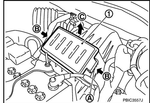
3. Remove air cleaner filter (1) and holder (2) assembly from the air cleaner case.
