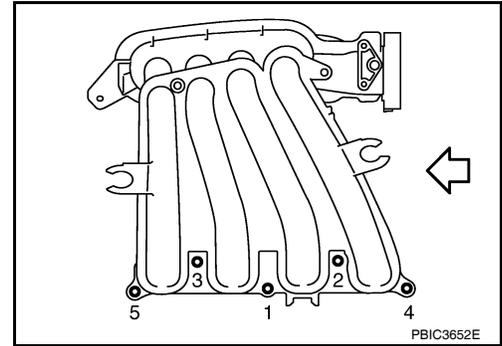
4. Install intake manifold support (front and rear).
