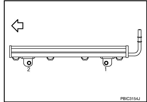
9. Remove the fuel tube and fuel injector assembly.
