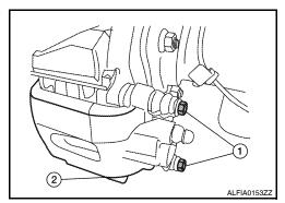
6. Apply matching marks to disc rotor and wheel hub assembly if the disc rotor is to be reused, then remove disc rotor.
