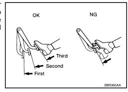
• Depress brake pedal while engine is running, and stop engine with pedal depressed. The pedal stroke should not change after holding pedal down for 30 seconds.
