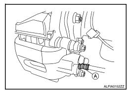
5. Remove sliding pin bolts (1) as shown, and remove cylinder body (2).
