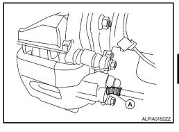
4. Refill with new brake fluid and bleed air. Refer to <a href="BR-17">BR-17</a>, "Bleeding Brake System".
