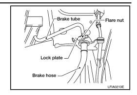
4. Remove union bolt and then remove brake hose from cylinder body.
