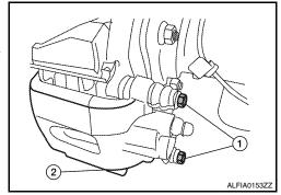
3. Install brake hose connection (A) and new copper washer to cylinder body and tighten to specification.
