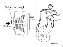
Output rod length [at -66.7 kPa (-500 mmHg, -19.69 inHg) vacuum] 15.6 - 15.9 (0.614 - 0.626)
