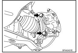
Apply matching marks to disc rotor and wheel hub assembly as shown if the disc rotor is to be reused, then remove disc rotor. CAUTION:
