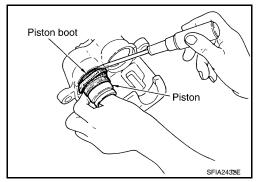
3. Apply clean brake fluid to pistons, then install pistons into cylinder body and insert piston boot side lip into groove of pistons as shown.
