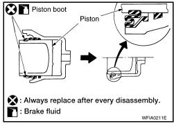
Insert into cylinder body by hand and insert piston boot piston-side lip into piston groove.
