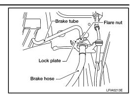
Remove brake hose connection (A) from cylinder body. NOTE:
