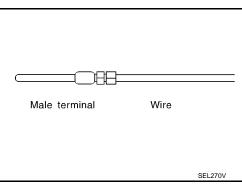
While holding the wire of the male terminal, try to insert the male terminal into the female terminal.
