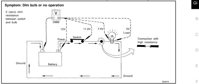
Measuring Voltage Drop — Steb-by-Step
