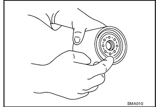
3. Screw the oil filter manually until it touches the installation surface, then tighten it by 2/3 turn. Or tighten to specification.
