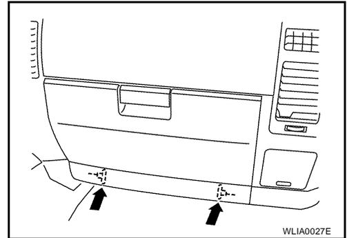
2. Remove the screw and remove the in-cabin microfilter cover.
