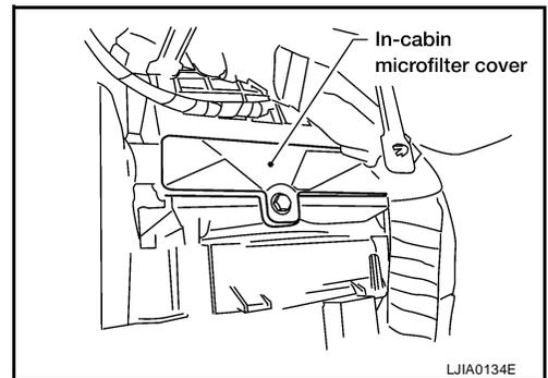
4. Insert the first new in-cabin microfilter into the front heater and cooling unit assembly housing and slide it over to the right. Insert the second new in-cabin microfilter into the front heater and cooling unit assembly housing.
