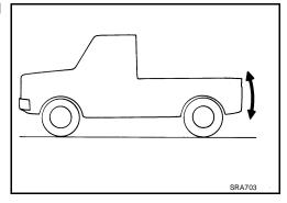
8. Tighten the rear spring shackle nuts, rear leaf spring front nut and shock absorber nuts to specification.
