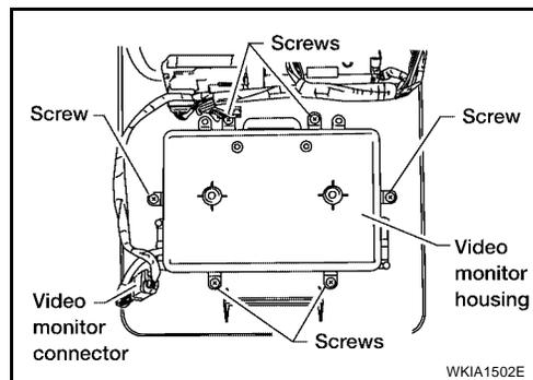
5. Remove the video monitor hinge screws and remove the video monitor.
