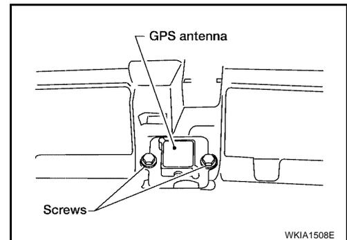
4. Disconnect GPS antenna connector and remove GPS antenna and feeder assembly out the top.
