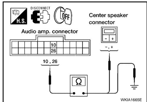
3. Check continuity between audio amp. harness connector M113 terminals and ground.
