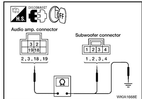
3. Check continuity between BOSE speaker amp. harness connector terminal and ground.
