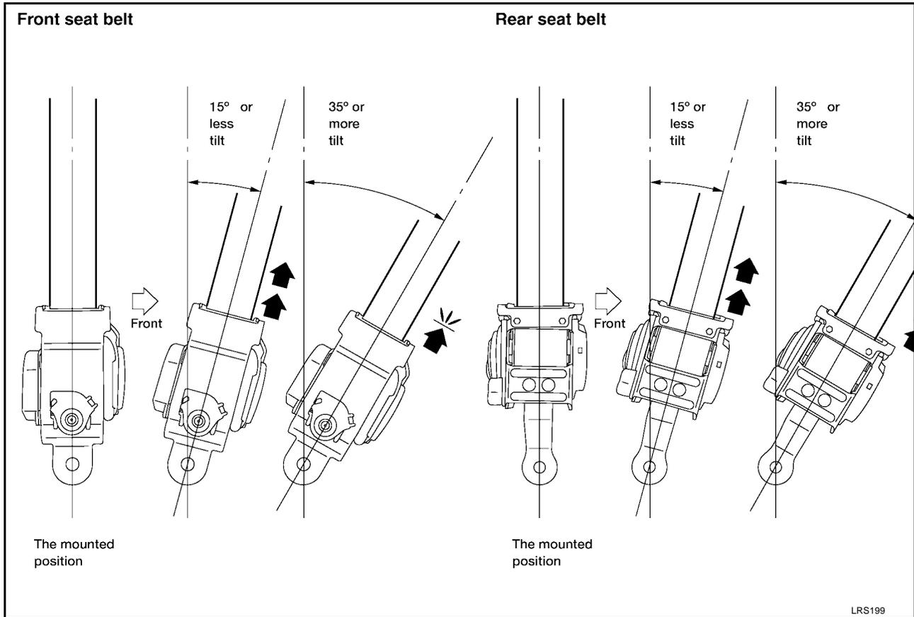
**15 degrees or less tilt : Belt can be pulled out.**
