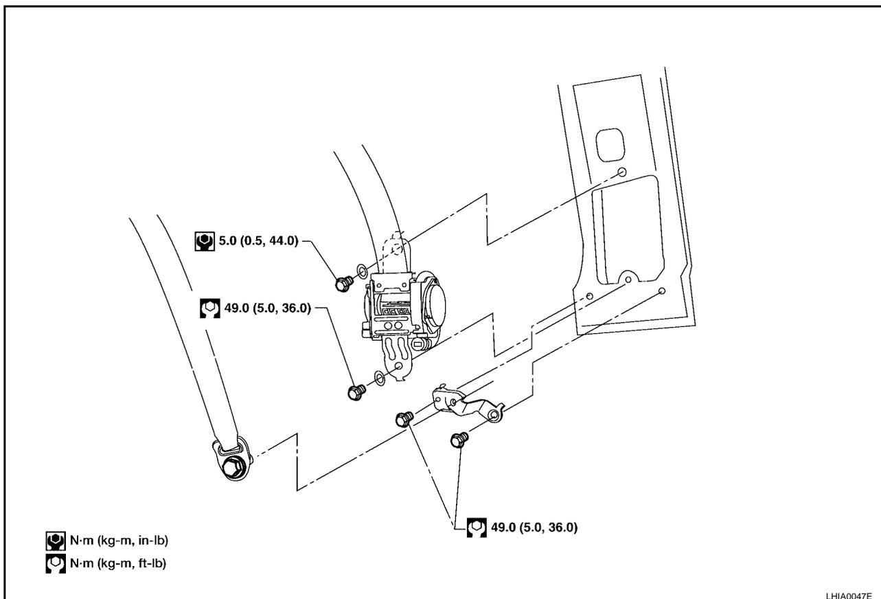
3. Disconnect the seat belt pre-tensioner electrical connector.
