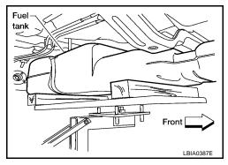
15. If necessary, remove the lock ring using Tool as shown.
