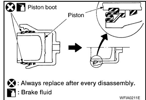
3. Insert piston into cylinder body by hand and insert piston boot piston-side lip into piston groove.
