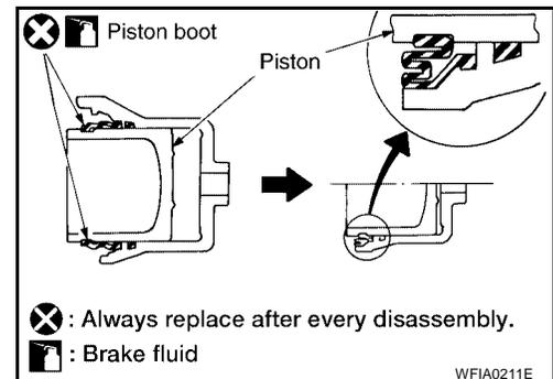
3. Insert into cylinder body by hand and insert piston boot piston-side lip into piston groove.
