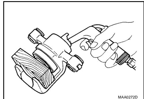
4. Using a flat-bladed screwdriver, remove piston seal from cylinder body.
