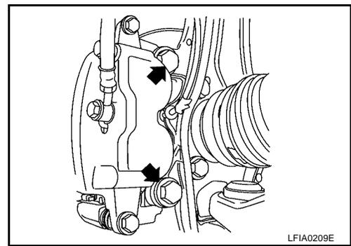
4. Install brake hose to brake caliper assembly, then tighten union bolt to the specified torque. Refer to [BR-23, "Components"](#).
