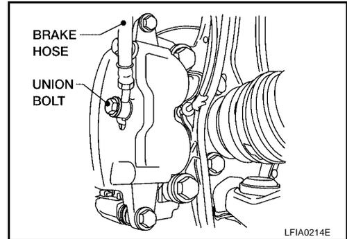
5. Refill new brake fluid and bleed air. Refer to [BR-11, "Bleeding Brake System"](#).
