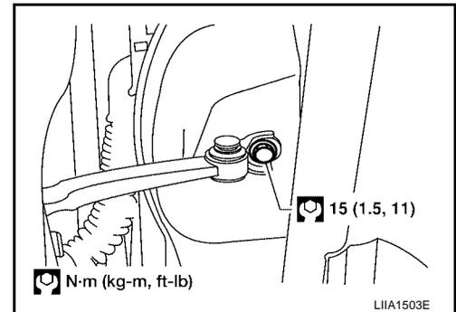
5. Remove the door-side hinge mounting nuts and bolts, and remove the door assembly.
