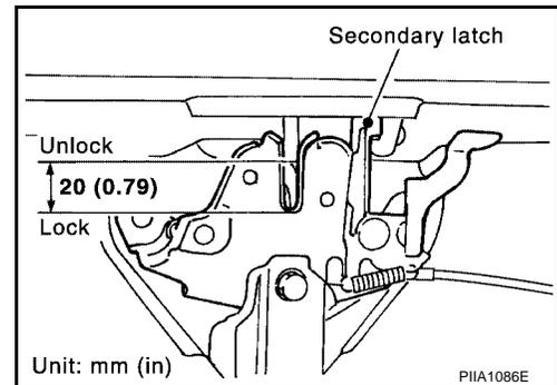
3. Check the hood lock lubrication condition. If necessary, apply body grease to the points shown in the figure.
