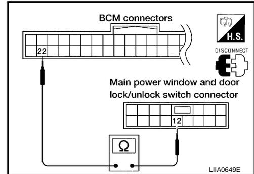
3. Check continuity between BCM connector M18 terminal 22 and power window and door lock/unlock switch RH connector D105 terminal 16.
