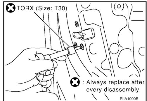
8. Remove the TORX bolt (T30) of the outside handle bracket.
