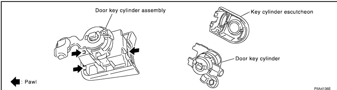
Remove the key cylinder escutcheon pawl and remove the door key cylinder.
