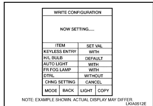
13. WRITE CONFIGURATION results are printed out automatically. Confirm "WRITE CONFIGURATION" is correctly executed by comparing sheet automatically printed out with applicable configuration list shown in step 9.
