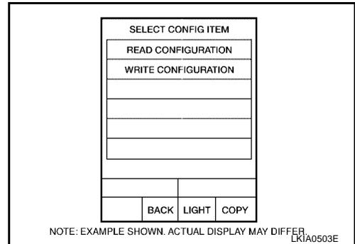
8. Configuration of current BCM is printed out automatically. A listing of manual setting items and auto setting items will be displayed. Auto setting items are preset and cannot be changed. Manual setting items can be set by using WRITE CONFIGURATION PROCEDURE. Refer to [BCS-16, "WRITE CONFIGURATION PROCEDURE"](#).
