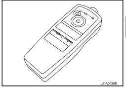
Register the IDs in order from FR LH, FR RH, RR RH and RR LH. When ID registration of each wheel has been completed, a buzzer sounds and the hazard warning lamps flash.
