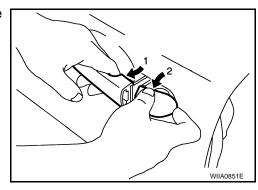
4. While pulling outside handle (1), slide toward rear of vehicle to remove (2).
