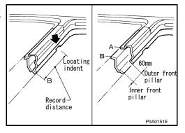
• Prepare a cutting jig to make outer pillar easier to cut. Also, this will permit service part to be accurately cut at joint position.
