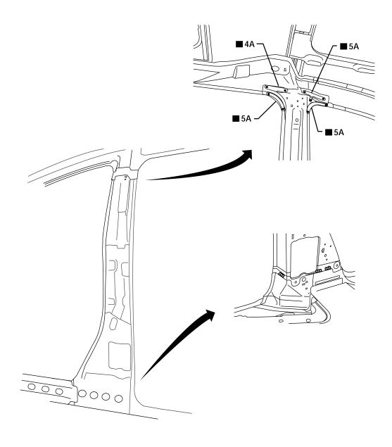
2-spot welds 3-spot welds MIG Plug weld
