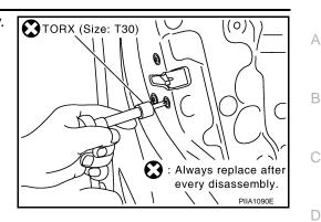
7. Remove the TORX bolt (T30), and remove the outside handle bracket.
