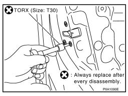
9. Remove the TORX bolt (T30) from the outside handle bracket.
