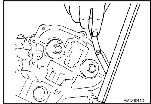
10. Install the IVT control solenoid valves with new gaskets.
