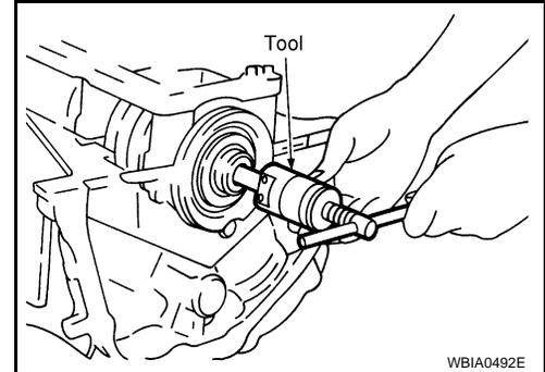
11. Cut away liquid gasket using Tool and remove rear oil seal retainer. Refer to [EM-4, "Precaution for Liquid Gasket"](#).
