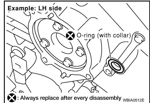
b. Install new seal rings on the IVT control covers.
