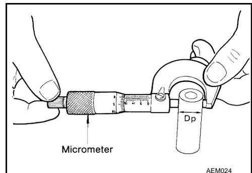
Piston and Piston Pin Interference Fit
