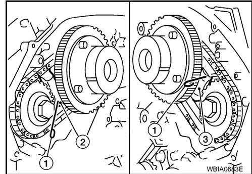
21. Remove the intake and exhaust camshaft sprocket bolts.
