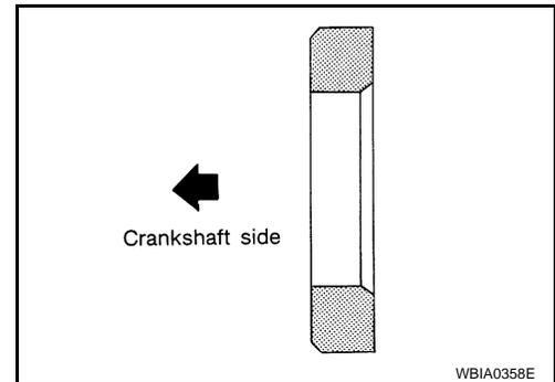
20. Install the drive plate and reinforcement plate aligning the matchmark.
