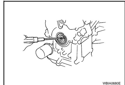
41. Remove O-rings and seal rings from front and rear timing chain case.
