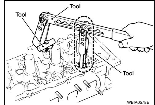
9. Install spark plug tube as follows:
