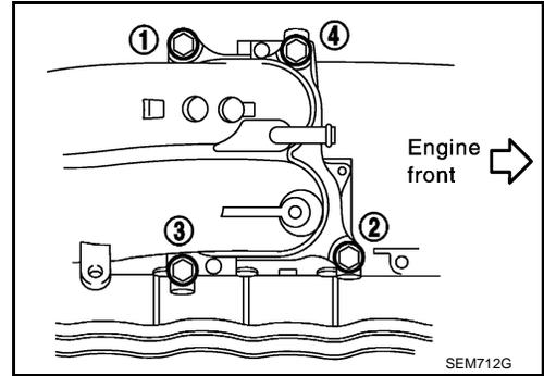
15. If necessary, remove power valve bolts in the order as shown and remove the power valve.
