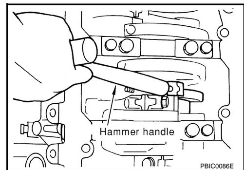
14. Remove the connecting rod bearings.
