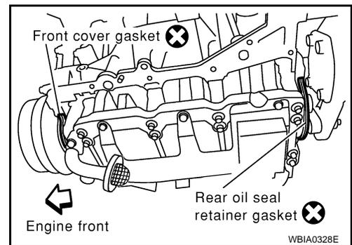
4. Apply a bead of sealant to the cylinder block mating surface of the upper oil pan as shown.
