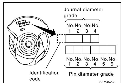
When Cylinder Block and Crankshaft are Reused
