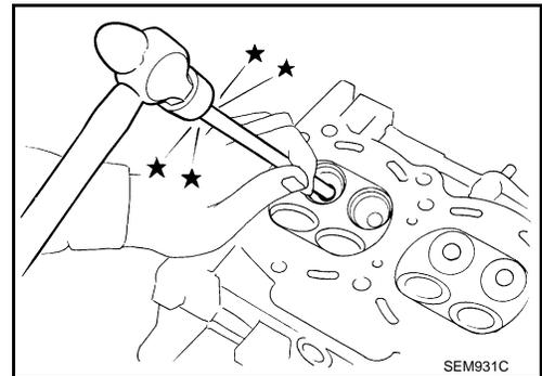
3. Ream cylinder head valve guide hole using suitable reamer.
