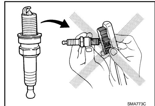
If plug tip is covered with carbon, a spark plug cleaner may be used.
