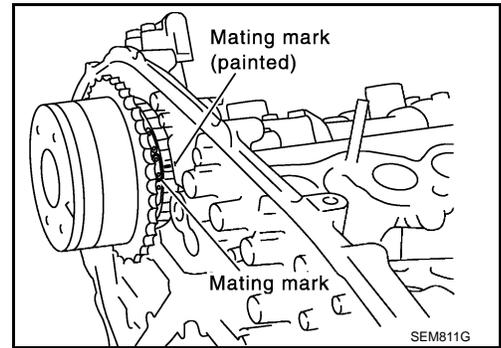
13. After confirming the mating marks are aligned, tighten the camshaft sprocket bolts.
