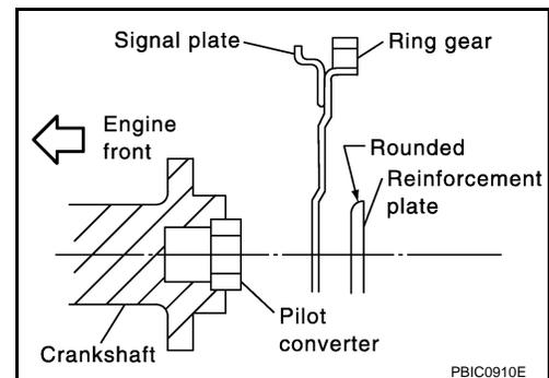
21. Secure the driveplate using Tool.
