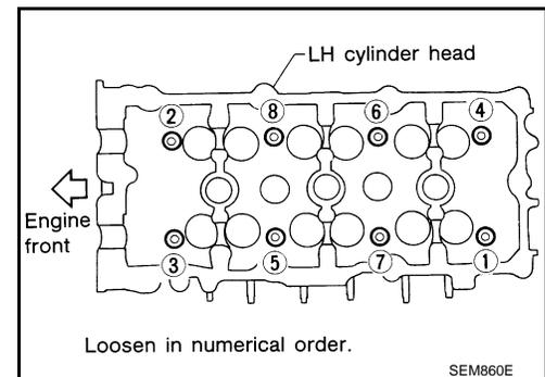
7. Remove cylinder heads and gaskets.
