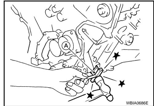
26. Remove the engine coolant inlet and thermostat assembly.
