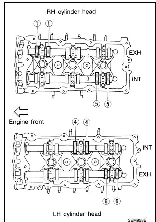
12. If all valve clearances are within specification, installation of the remaining components is in the reverse order of removal. If the valve clearances are out of specification, adjust the valve clearances. Follow the "VALVE ADJUSTING" procedure.
