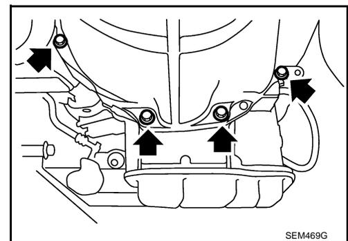
8. Apply a continuous bead of sealant to the lower oil pan.
