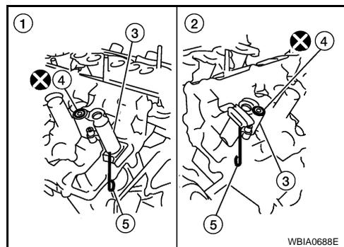
9. Install exhaust and intake camshafts and camshaft brackets.
