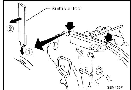
c. Use the Tool by tapping (1) and sliding (2) using a plastic hammer to remove the lower oil pan from the upper oil pan.
