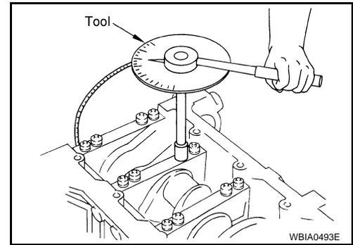
e. After tightening the bearing cap bolts, make sure the crankshaft turns smoothly.
