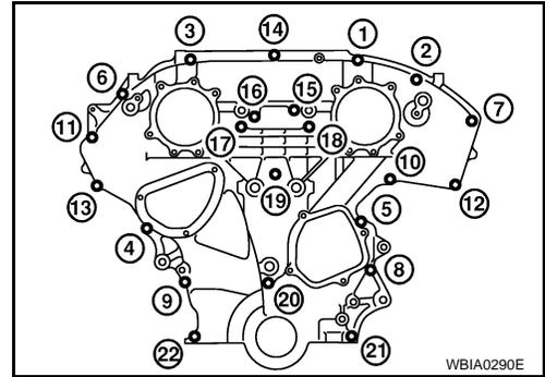
b. Insert the suitable tool into the notch (1) at the top of the front timing chain case to pry (2) it loose as shown.
