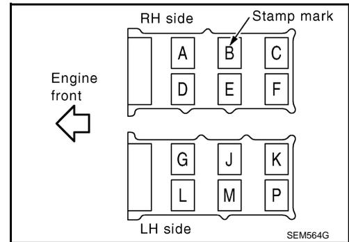
8. Tighten the camshaft brackets in the four steps, as shown.
