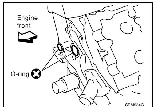
15. Install RH (1) and LH (2) new O-rings (3) on the cylinder heads.
