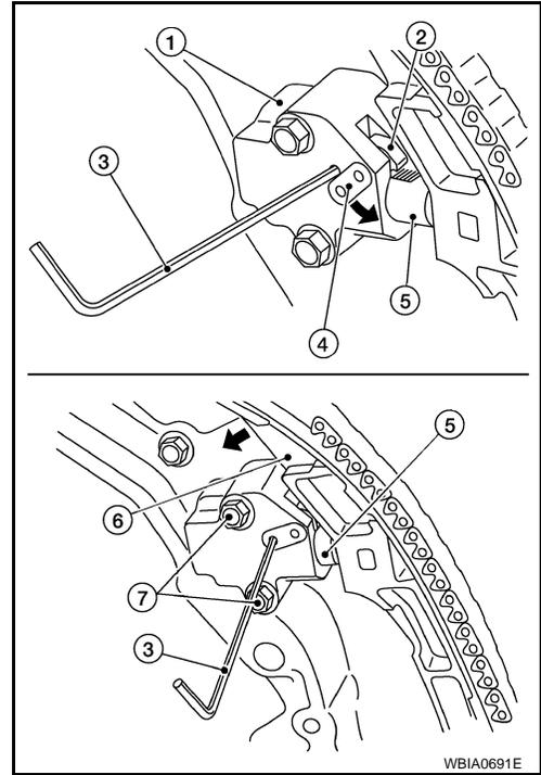
19. Remove primary timing chain and crankshaft sprocket.
