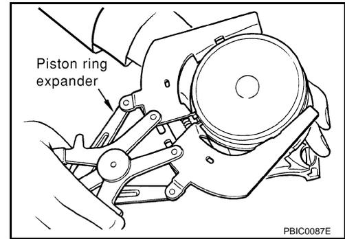
16. Remove the piston from the connecting rod as follows.
