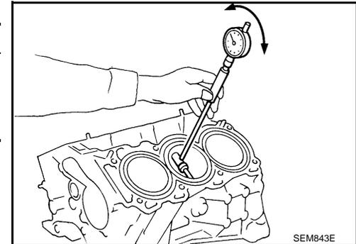
If it exceeds the limit, re bore all cylinders. Replace cylinder block if necessary.
