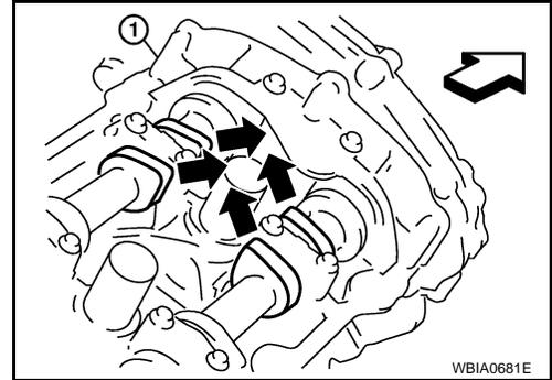
14. Lock the ring gear using Tool attached to the starter bolt hole.
