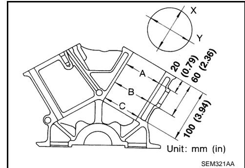
5. Determine piston oversize according to amount of cylinder wear.
