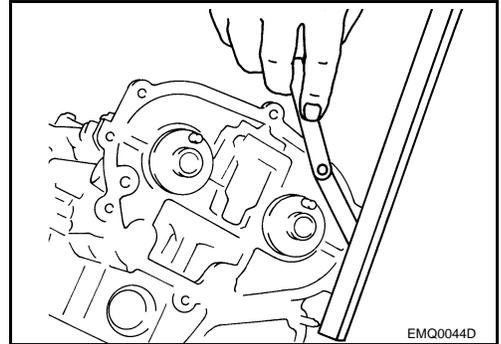
13. Install the IVT control solenoid valves with new gaskets.
