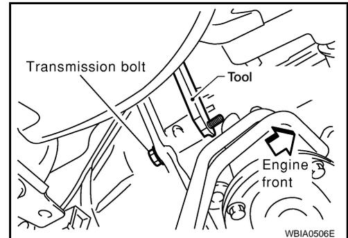
36. Rotate crankshaft pulley in normal direction (clockwise when viewed from front) to confirm it turns smoothly.
