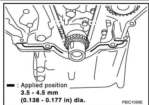
6. Install front timing chain case.
