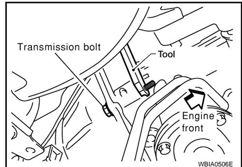
15. Remove the crankshaft pulley as follows:
