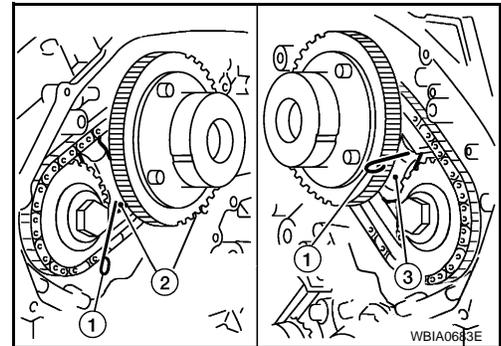
15. Install the crankshaft sprocket on the crankshaft.
