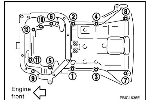
7. Install the four upper oil pan to transaxle bolts. Refer to [EM-110. "Removal and Installation"](#).
