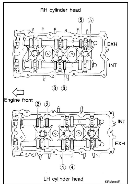
9. Turn the crankshaft 240° and align as above.
