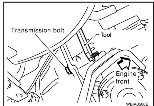
31. Remove the crankshaft pulley as follows:
