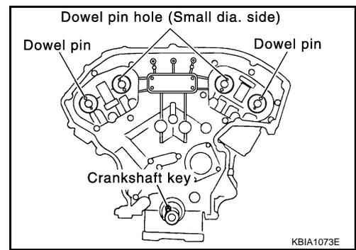
12. Install the secondary timing chains and camshaft sprockets.
