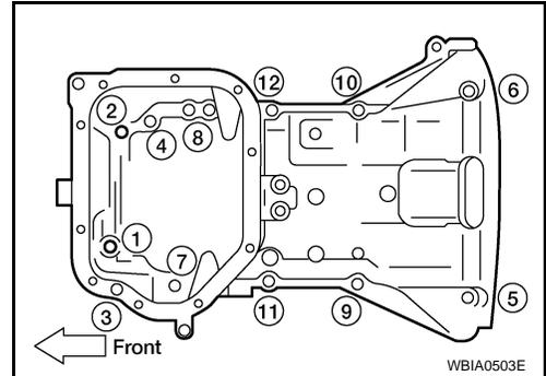
b. Insert a suitable tool into the notch (1) of the upper oil pan as shown.
