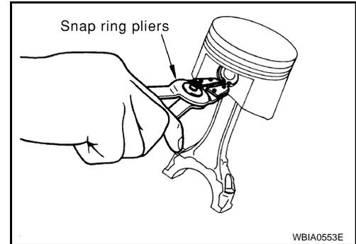
b. Heat the pistons to 60° - 70°C (140° - 158°F).
