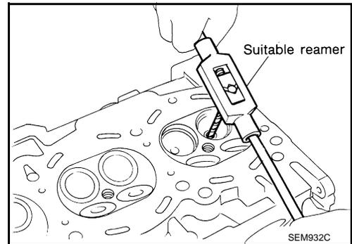
4. Heat cylinder head to 110° - 130°C (230° - 266°F) by soaking in heated oil and press new valve guide from camshaft side into the cylinder head to the dimensions as shown.
