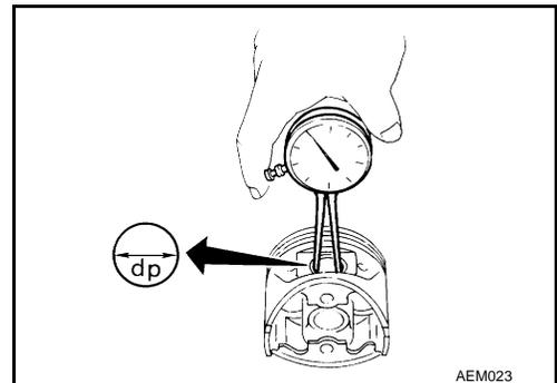
Outer Diameter of Piston Pin
