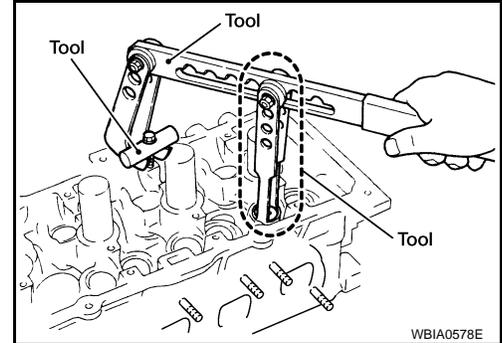
4. Remove valve oil seal using Tool.
