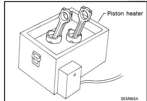
c. Push out the piston pin using a suitable tool, with an outer diameter approximately 20 mm (0.8 in).
