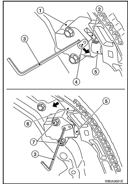
20. Reconfirm that the matching marks on the sprockets and the timing chain have not slipped out of alignment.
