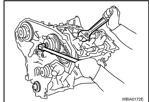
14. Pull the stopper pins (1) out from the secondary timing chain tensioners (2) and (3).
