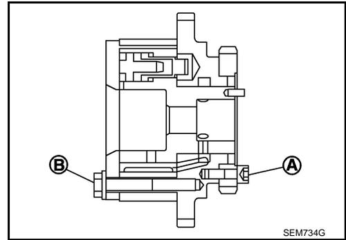
23. Loosen the No. 1 camshaft bracket bolts in several steps in the order as shown and remove No. 1 camshaft brackets.
