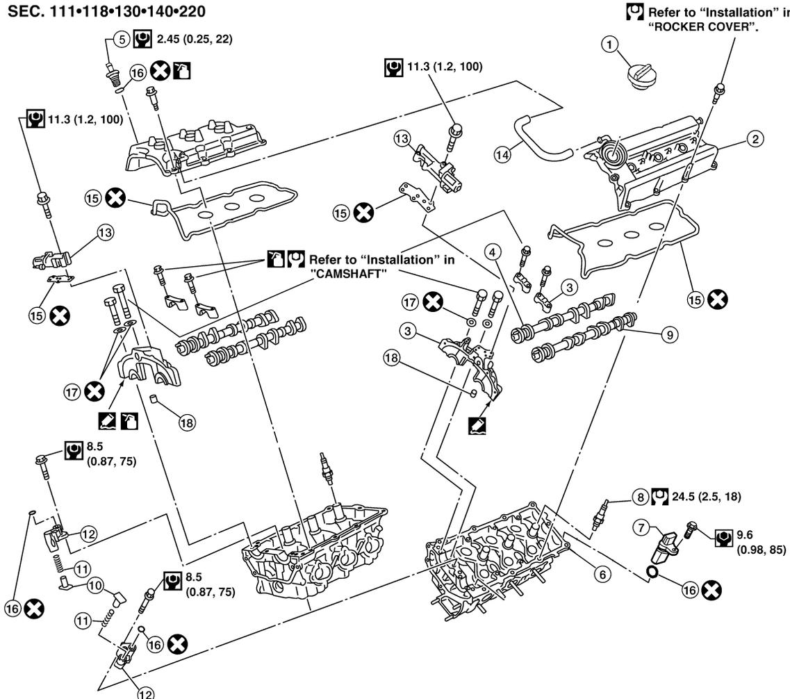
: Apply Genuine Silicone RTV Sealant or equivalent.
