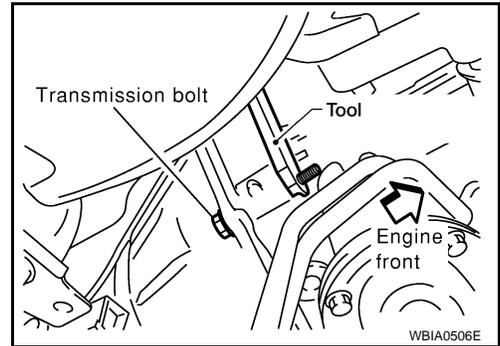
4. Rotate crankshaft pulley in normal direction (clockwise when viewed from front) to confirm it turns smoothly.
