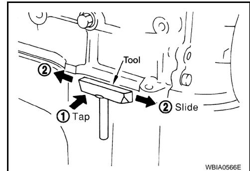
38. Remove the water pump cover and chain tensioner cover from the front timing chain case using Tool.
