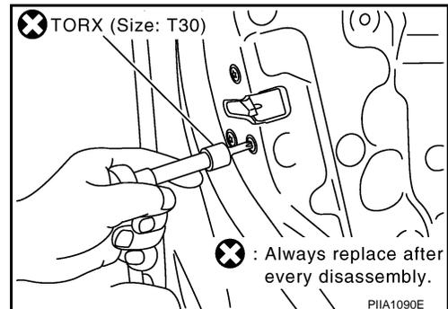
9. Remove the TORX bolt (T30) from the outside handle bracket.
