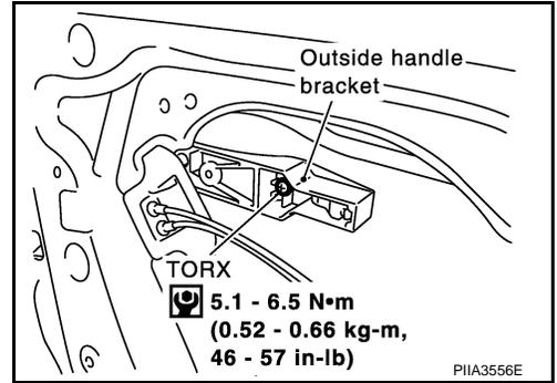
8. While pulling outside handle, slide toward rear of vehicle to remove outside handle and door lock assembly.
