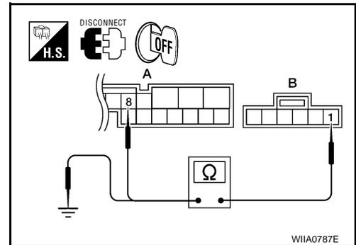
3. Check continuity between back door close switch connector (B) B63 terminal 1 and ground.
