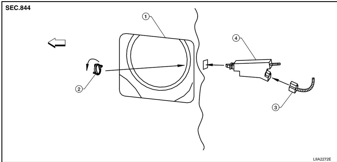
1. Fuel filler lid opening (LH rear fender) 2. Lock ring 3. Electrical connector
