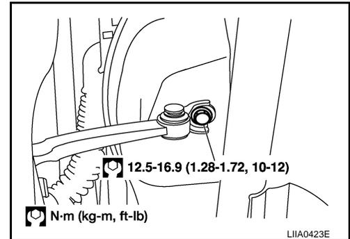
5. Remove the door-side hinge nuts and bolts, and remove the door assembly.
