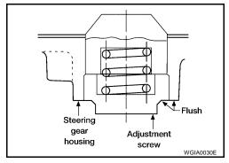
2. Loosen adjusting screw in  $40^{\circ}$  -  $60^{\circ}$  increments until rack sliding force is within specification.
