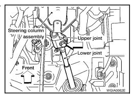
Remove nuts from steering member, remove steering column assembly from steering member.
