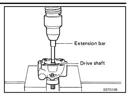
Remove oil seal for body assembly, using a suitable tool.
