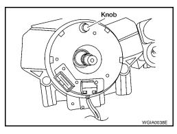
Tighten steering wheel center nut to specification. Refer to <u>PS-9</u>, "Removal and Installation".
