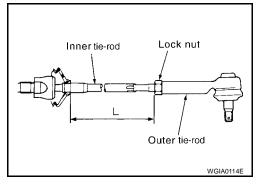
Measure rack stroke. Refer to <u>PS-29</u>, "<u>Steering Gear and Link-age</u>".
