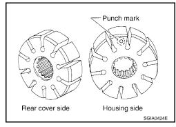
Install vane to rotor with arc of vane in contact with cam ring.
