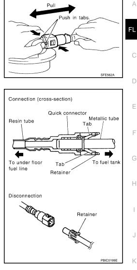
Visually confirm that the two retainer tabs are connected to the quick connector.
