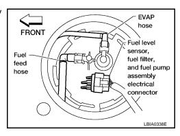
Turn the lock ring until the lock ring is fully rotated into the fuel tank lock tabs as shown.
