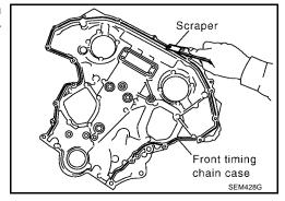
41. Remove all old Silicone RTV Sealant from all the bolt holes and bolts.
