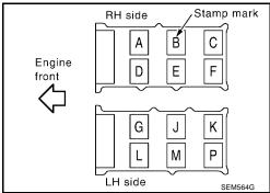
8. Tighten the camshaft brackets in the four steps, in the order as shown.
