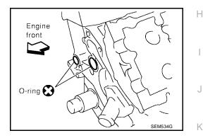
15. Install RH (1) and LH (2) new O-rings (3) on the cylinder heads.
