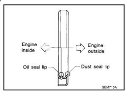
Press in rear oil seal to the position as shown.
