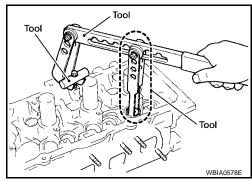
Remove valve oil seal using Tool.
