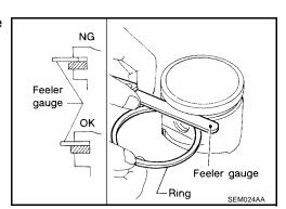
If out of specification, replace piston ring assembly. If clearance exceeds maximum limit with new rings, replace piston
