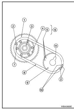
It may be difficult to visually check the dislocation of mating marks during and after installation. To make the matching easier, make a mating mark on the sprocket teeth in advance with paint.
