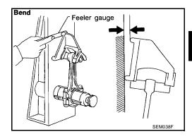
If it exceeds the limit, replace connecting rod assembly.
