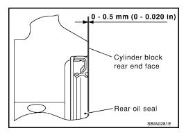
Press-fit rear oil seal using Tool.
