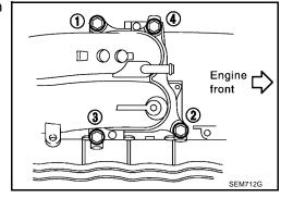
If necessary, install the electric throttle control actuator bolts in the order as shown. Install gasket with three protrusions facing down.
