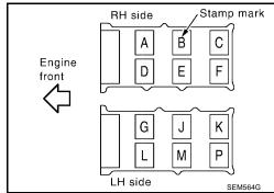
11. Tighten the camshaft brackets in four steps in the order as shown.
