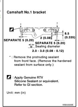
3. Tighten the No. 1 camshaft bracket in three steps, in the order as shown.
