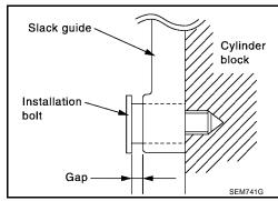
19. Install the timing chain tensioner (1) and slack guide (6).
