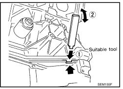
23. Remove the O-ring seals from the bottom of the cylinder block and oil pump housing, use new O-rings for installation.
