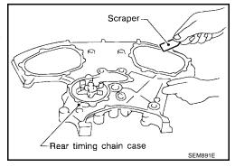
Remove the old Silicone RTV Sealant from the bolt hole and thread.
