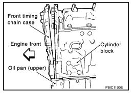
b. While pressing front timing chain case from its front and top as shown, hammer dowel pin until the outer end becomes flush with surface using suitable tool.
