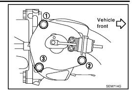
If necessary, tighten the intake manifold collector (upper) bolts in the order as shown.
