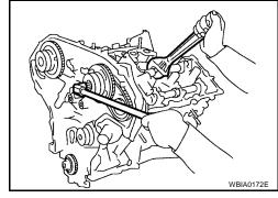
14. Pull the stopper pins (1) out from the secondary timing chain tensioners (2) and (3).
