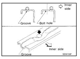
5. Install new O-rings on the cylinder block and oil pump body.
