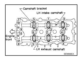
12. Measure difference in levels between front end faces of camshaft No. 1 bracket and cylinder head.
