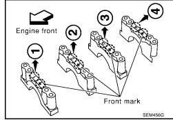
d. Tighten the bearing cap bolts in two steps in the order as shown:
