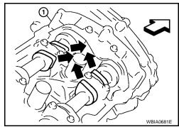
24. Lock the ring gear using Tool attached to the starter bolt hole.
