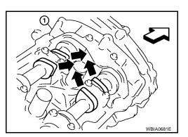
14. Lock the ring gear using Tool attached to the starter bolt hole.
