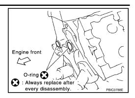
28. If necessary, remove the water pump. Refer to <u>CO-17</u>, <u>"REMOVAL"</u>.
