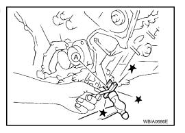
37. Remove O-rings (3) on the RH (1) and LH (2) No.1 camshaft bracket, cylinder head and cylinder block.
