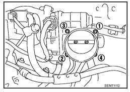
• Install the intake manifold collector (lower) bolts in the order as shown.
