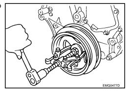
3. Remove front oil seal from front timing chain case.
