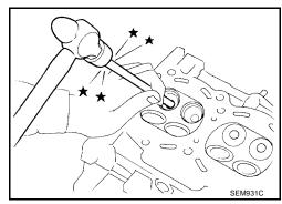
Ream cylinder head valve guide hole using suitable reamer.
