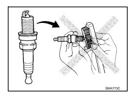
If plug tip is covered with carbon, a spark plug cleaner may be used.
