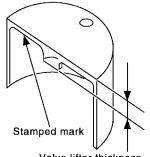
Valve lifter thickness
