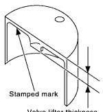
Valve lifter thickness
