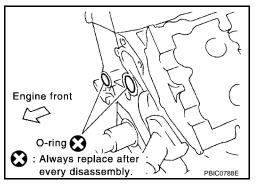
Install new O-rings (3) on the RH (1) and LH (2) cylinder heads.
