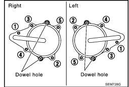
28. Apply liquid gasket and install the chain tensioner cover.
