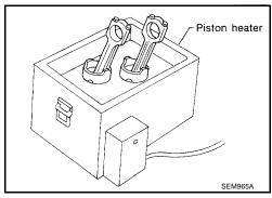
c. Push out the piston pin with a suitable tool, with an outer diameter approximately 20 mm (0.8 in).
