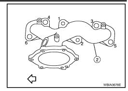
Install the RH (1) and LH (2) three way catalyst support bolts in the order as shown.
