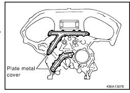
Loosen and remove the rear timing chain case bolts in the order as shown.
