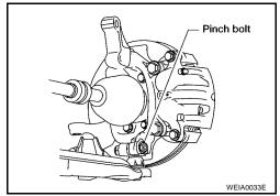
28. Disconnect the connecting rod from the front strut using power tool.
