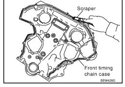
31. Remove all old Silicone RTV Sealant from all the bolt holes and bolts.
