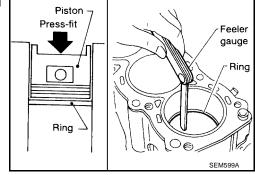
If out of specification, replace piston ring. If gap still exceeds the limit even with a new ring, re-bore cylinder and use oversized piston and piston ring.
