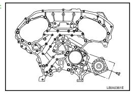
7. Apply Silicone RTV Sealant to rear timing chain case as shown.
