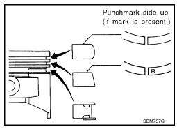
Position each ring with the gap as shown, referring to the piston front mark.
