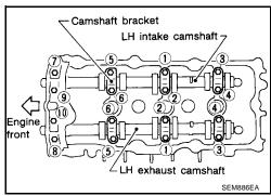
Measure difference in levels between front end faces of No.1 camshaft bracket and cylinder head.
