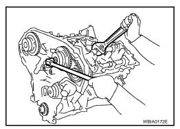
22. Remove the secondary timing chains (3) with camshaft sprockets.
