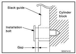
19. Install the timing chain tensioner (1) and slack guide (6).
