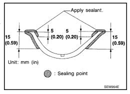
3. Install a new front cover gasket and rear oil seal retainer gasket.
