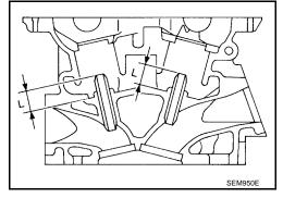
5. Apply a reamer finish to the valve guide, using suitable reamer.
