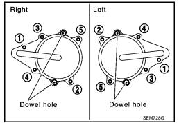
28. Apply liquid gasket and install the chain tensioner cover.
