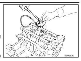
Install pilot converter as shown.
