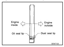
Make sure the garter spring is in position and seal lip is not inverted.
