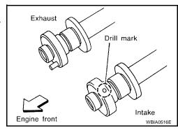
• Follow your identification marks (2) and (3) made during removal, or follow the identification marks (1) that are present on the new camshafts components for proper placement and direction of the components.
