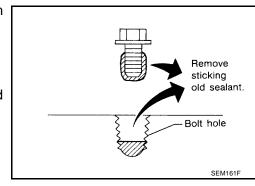
Before installing the No. 1 camshaft bracket, remove the old Silicone RTV Sealant from the mating surface using suitable scraper.
