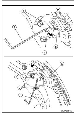
29. Remove primary timing chain and crankshaft sprocket.
