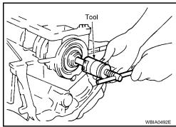
12. Cut away liquid gasket using Tool and remove rear oil seal retainer. Refer to EM-4, "REMOVAL OF LIQUID GASKET SEALING".
