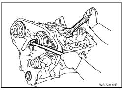
14. Pull the stopper pins (1) out from the secondary timing chain tensioners (2) and (3).
