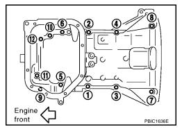
7. Install the four upper oil pan to transaxle bolts. Refer to <a href="EM-135">EM-135</a>, <a href=""">"INSTALLATION"</a>.
