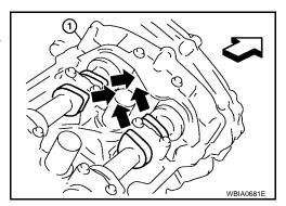
30. Lock the ring gear using Tool attached to the starter bolt hole.
