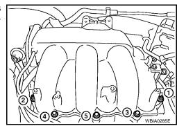
13. If necessary, remove the electric throttle control actuator bolts in the order as shown and remove the electric throttle control actuator.
