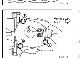
• If necessary, install power valve bolts in the order as shown.
