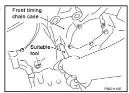
7. Loosely install the front timing chain case bolts.
