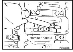
15. Remove the connecting rod bearings.
