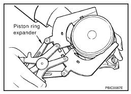
When replacing the piston rings, those without punch marks can be mounted either side up.
