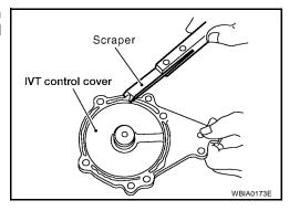
43. Remove the old Silicone RTV Sealant from the camshaft No. 1 bracket mating surface using a scraper.
