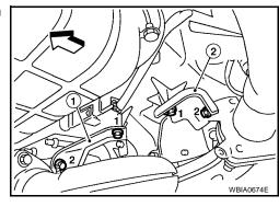
Install the exhaust manifold heat shield bolts.
