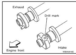
• Follow your identification marks made during removal, or follow the identification marks that are present on the new camshaft components for proper placement.
