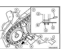
• Do not disassemble the intake sprockets (never loosen bolts A and B as shown).
