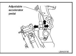
Check the accelerator pedal for smooth operation. There should be no binding or sticking when applying
