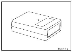
7. Register the IDs in order from FR LH, FR RH, RR RH and RR LH. When ID registration of each wheel has been completed, a buzzer sounds and the hazard warning lamps flash.
