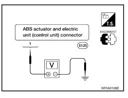
2. Check resistance between ABS actuator and electric unit (control unit) connector E125 and ground.
