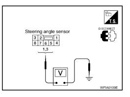
3. Check resistance between steering angle sensor connector M47 and ground.
