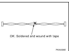
• Do not make a bypass connection to repaired area. (If the circuit is bypassed, characteristics of twisted wire will be lost.)
