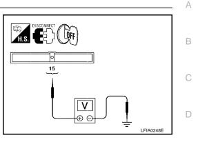
2. Check resistance between ABS actuator and electric unit (control unit) connector E125 and body ground.
