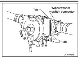
8. While pressing tabs, pull lighting and turn signal switch toward driver door and disconnect from base.
