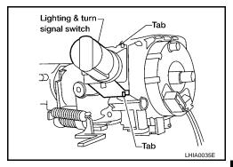
9. Remove the screws, release the tab, and remove the spiral cable.
