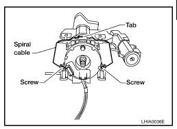
10. Remove the spiral cable connectors.
