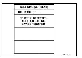
"SELF-DIAG [PAST]" Return to the "SELF-DIAG [CURRENT]" CONSULT-II screen by touching "BACK" key of CONSULT-II and select "SELF-DIAG [CURRENT]" in SELECT DIAG MODE. Touch "ERASE" in "SELF-DIAG [CURRENT]" mode.
