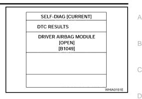
If no malfunction is detected on "SELF-DIAG [CURRENT]" even though malfunction is detected in "SRS Operation Check", refer to SRS-30, "DIAGNOSTIC PROCEDURE 4 (CONTINUED FROM DIAGNOSTIC PROCEDURE 2)", to diagnose the following cases:
