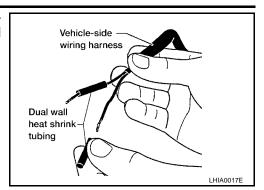
Fold each wire back and insert into the end of the heat shrink tubing so that the end of the wire is approximately centered in the heat shrink tubing.
