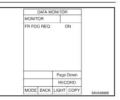
Start auto active test. Refer to <u>PG-21, "Auto Active Test"</u>. When front fog lamp relay is operating, check voltage between left/right front fog lamp connector terminals and ground.
