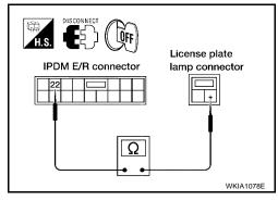
5. Check continuity between IPDM E/R harness connector and rear combination lamp harness connector.
