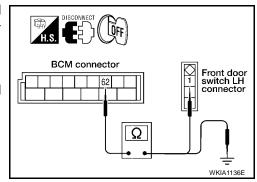
Check continuity between front door switch LH terminal 1 and exposed metal of switch while pushing and releasing switch.
