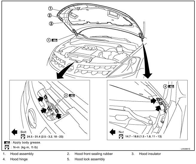
1. Support the hood striker with a proper material to prevent it from falling.
