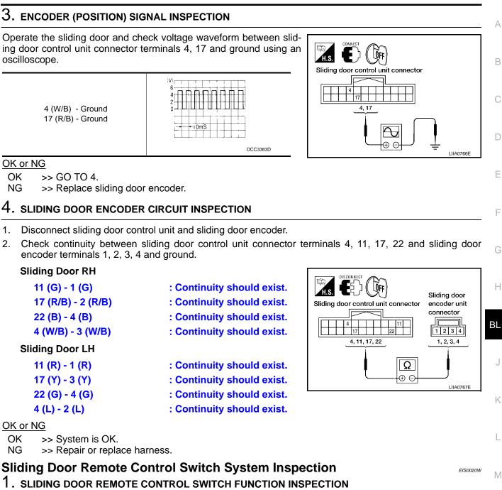
Check sliding door remote control switch operation.
