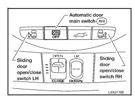
4. Within 3 seconds after step 3, press the door pillar Sliding Door Open/Close Switch of the door being initialized 10 times within 10 seconds.
