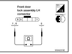
NG >> Replace front door lock assembly LH. Refer to <u>BL-166, "FRONT DOOR LOCK"</u>.
