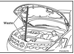
2. Remove the hinge nuts on the hood to remove the hood assembly.
