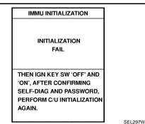
INITIALIZATION FAIL THEN IGN KEY SW 'OFF' AND 'ON', AFTER CONFIRMING SELF-DIAG AND PASSWORD, PERFORM C/U INITIALIZATION AGAIN.
