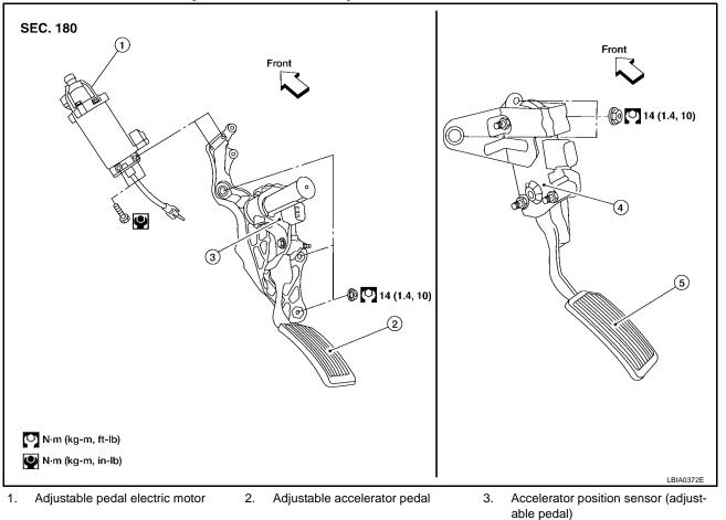
4. Accelerator position sensor (non- 5. Non-adjustable accelerator pedal adjustable pedal)
