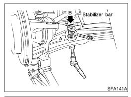
When removing or installing stabilizer bar, secure portion A with wrench as shown.
