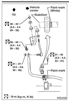
When installing stabilizer, it must be positioned as shown.
