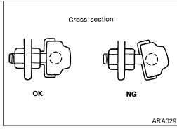
Install stabilizer bar with ball joint socket properly placed.
