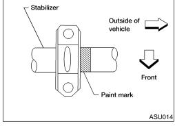
When installing stabilizer, make sure that paint mark and clamp are in the correct positions.
