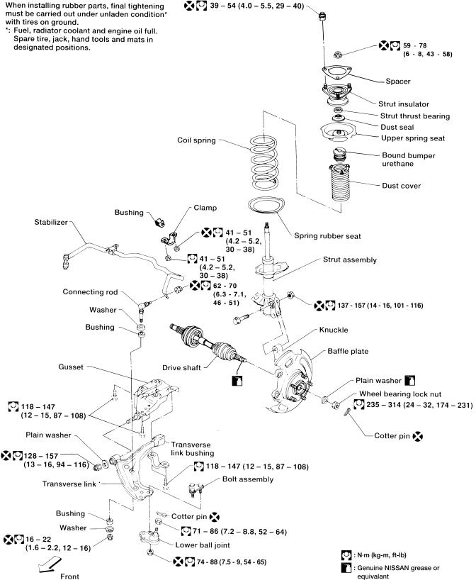
Coil Spring and Strut Assembly (Cont'd)
