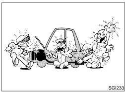
To prevent serious burns: Avoid contact with hot metal parts. Do not remove the radiator cap when the engine is hot.
