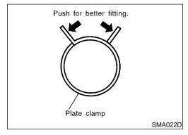
After installing leaf spring clamps, apply force to them in the direction of the arrows, tightening rubber hose equally all around.
