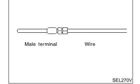
While holding the wire of the male terminal, try to insert the male terminal into the female terminal.
