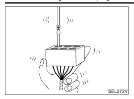
While moving the connector, check whether the male terminal can be easily inserted or not.
