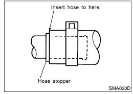
To reinstall the rubber hose securely, make sure of hose insertion length and clamp orientation. (If tube is equipped with hose stopper, insert rubber hose into tube until it butts up against hose stopper.)
