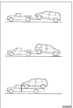
Nissan recommends that the vehicle be towed with the driving (front) wheels off the ground as illustrated.
