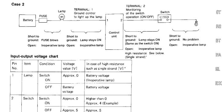
The voltage value is based on the body ground.
