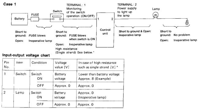
The voltage value is based on the body ground.
