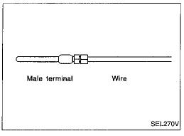
Assemble a male terminal and approx. 10 cm (3.9 in) of wire.
