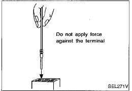
While holding the wire of the male terminal, try to insert the male terminal into the female terminal.
