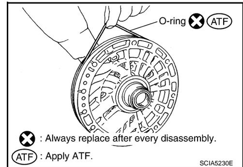
2. Install O-ring to oil pump housing.
