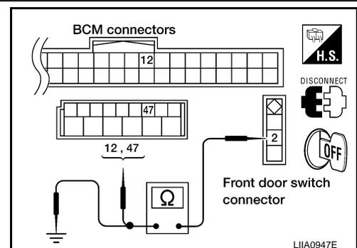
4. Check continuity between front door switch connector and ground.
