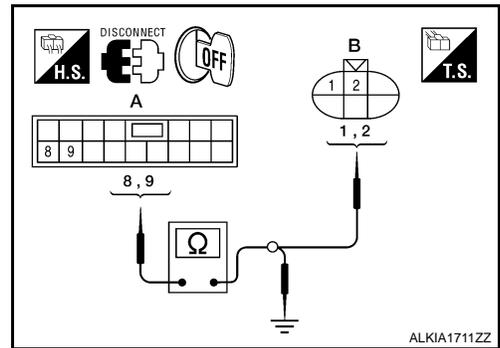
4. Check continuity between power window and door lock/unlock switch RH connector (A) and ground.
