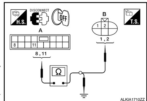
4. Check continuity between main power window and door lock/unlock switch connector (A) and ground.
