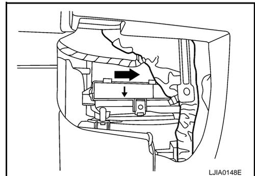
5. Install the in-cabin microfilter cover.
