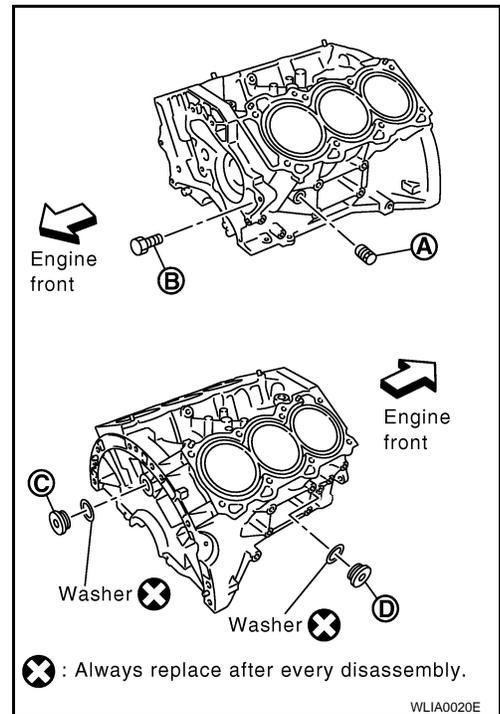
Block Plug and Block Heater Installation
