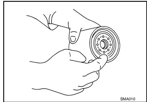
3. Screw on the oil filter manually until it touches the installation surface, then tighten it by 2/3 turn as shown. Or tighten to specification.
