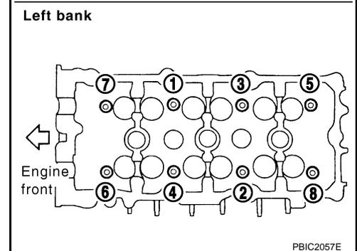
Measure the tightening angle using Tool.
