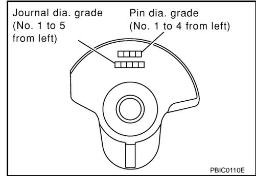
3. Read the symbol at the cross point of the selected row and column in the "Main Bearings Selection Table".
