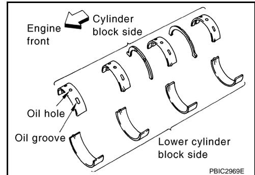
5. Install crankshaft to cylinder block.
