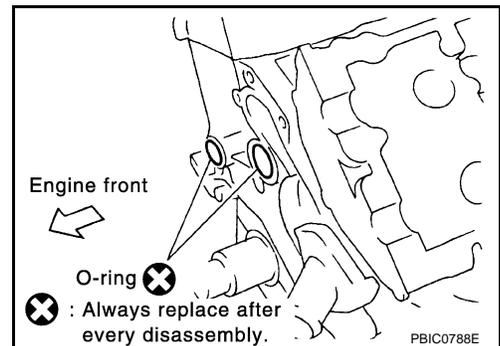
32. Remove timing chain tensioners (secondary) from cylinder head if necessary.
