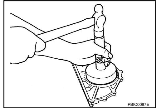
9. Install rear oil seal retainer.
