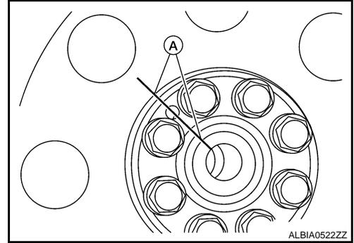
3. Lock the drive plate using Tool (A).
