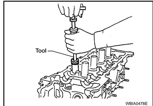
8. Replace the valve seat if necessary. Refer to [EM-214, "Inspection After Disassembly"](#).
