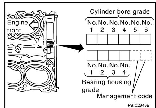
When Cylinder Block is Reused
