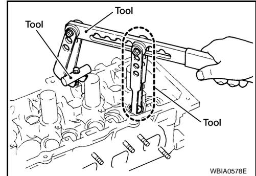
9. Install the valve lifters.
