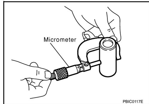
Connecting Rod Bushing Oil Clearance (Small End)
