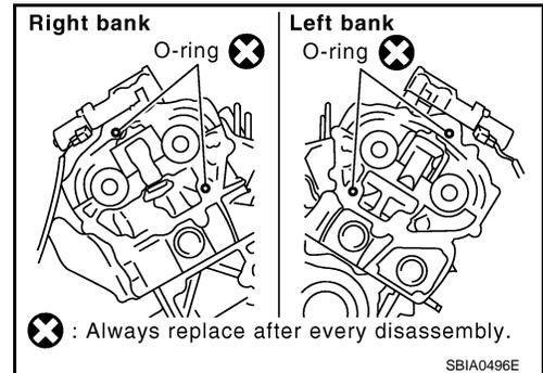
31. Remove O-rings from cylinder block.
