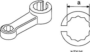
Loosening or tightening heated oxygen sensor 1<br>a: 22 mm (0.87 in)<br>NT636                                                   |
