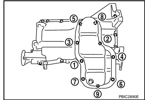
2. Install oil pan drain plug. Refer to [EM-35, "Removal and Installation"](#).
