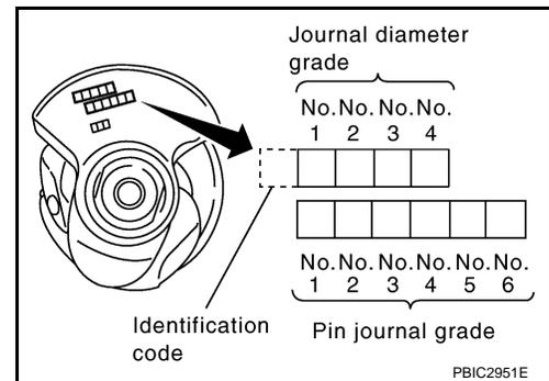
When Crankshaft and Connecting Rod are Reused
