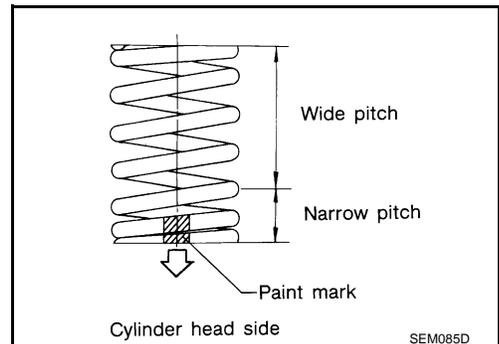
7. Install valve spring retainer.
