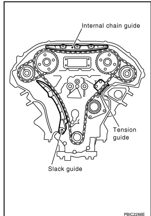
26. Remove timing chain (primary) and crankshaft sprocket.
