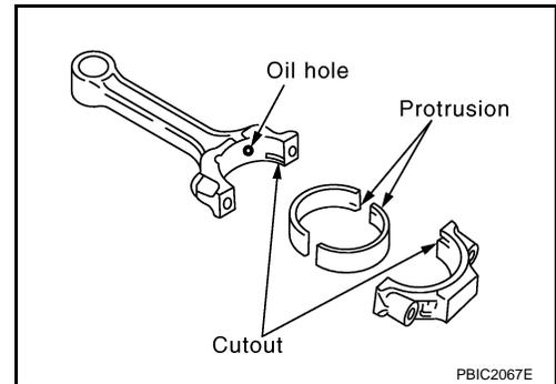
12. Install piston and connecting rod assembly to crankshaft.
