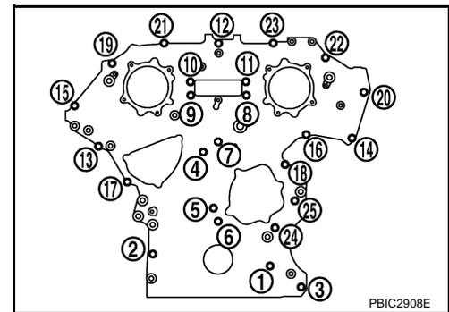
5. Install two bolts in front of oil pan (upper) in numerical order as shown.
