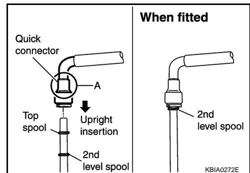
4. Pull quick connector by hand holding (A) position. Make sure it is completely engaged (connected) so that it does not come out from fuel tube.
