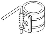
Installing piston assembly into cylinder bore                                                                                                                                                        | I<br>J<br>K  |
