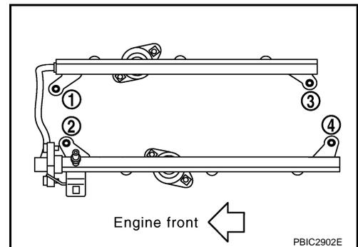
6. Remove bolts which connects fuel tube (RH) and fuel tube (LH).
