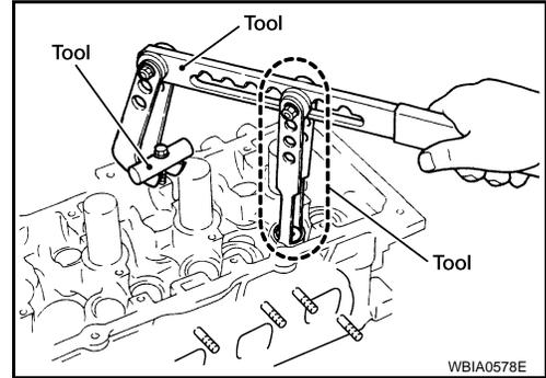
5. Remove valve oil seal using Tool.
