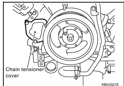
7. Remove the chain tensioner (RH) using the following steps.
