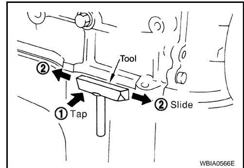
3. Remove the oil cooler assembly. Refer to [LU-28. "Removal and Installation"](#).
