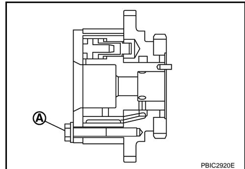
28. Remove water pump. Refer to [CO-22](#). "Removal and Installation".
