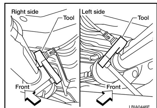
5. Remove center exhaust tube, main muffler and left front exhaust tube. Refer to [EX-6, "Removal and Installation"](#).
