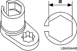
Loosening or tightening air fuel ratio A/F sensor<br>a: 22 mm (0.87 in)<br>LBIA0444E                                            |
