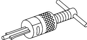
Removing crankshaft pilot bushing                                                                                                                                                                    | N<br>O       |
