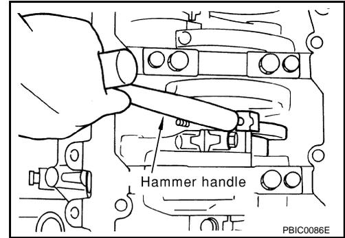
8. Remove connecting rod bearings.
