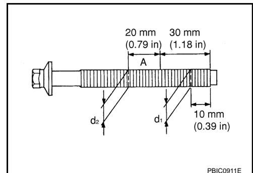
**CONNECTING ROD BOLT OUTER DIAMETER**
