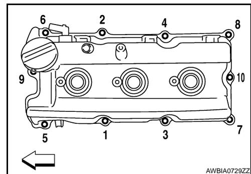
5. Install the oil filler cap to rocker cover (LH), if removed.
