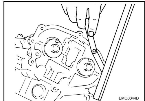
7. Check and adjust the valve clearance. Refer to [EM-18, "Valve Clearance"](#).
