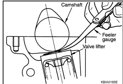
8. Turn the crankshaft pulley clockwise 270° from the position of No. 1 cylinder compression TDC to obtain No. 3 cylinder compression TDC.
