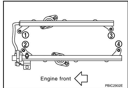
6. Tighten bolts which connects fuel tube (RH) and fuel tube (LH) to the specified torque.
