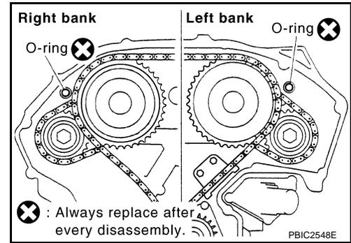
Fit lower end of front timing chain case tightly onto top face of oil pan (upper). From the fitting point, make entire front timing chain case contact rear timing chain case completely.
