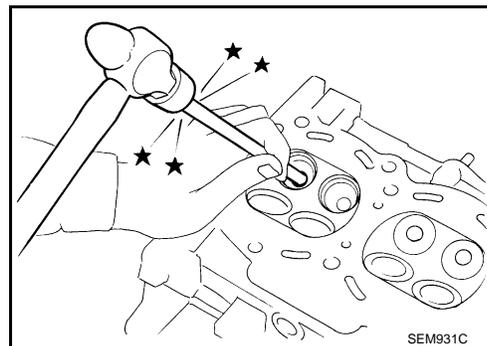
3. Ream cylinder head valve guide hole using suitable tool.
