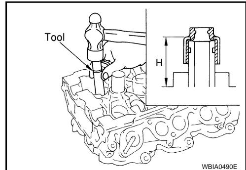
6. Install valve spring (uneven pitch type).
