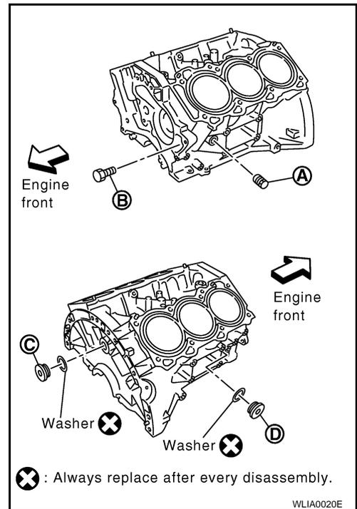
Block Plug and Block Heater Installation
