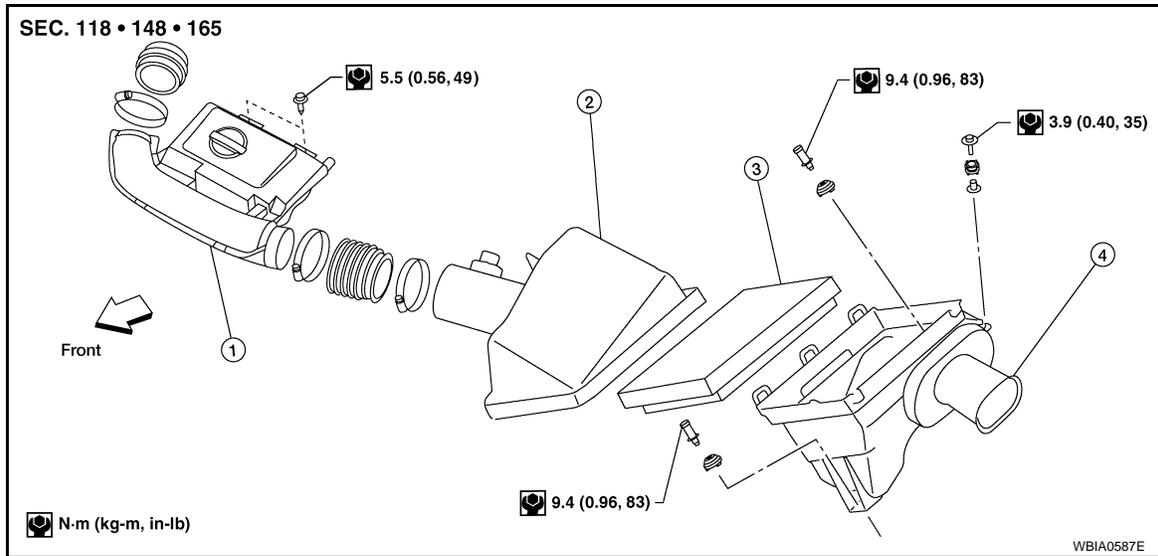
1. Air duct and resonator assembly
