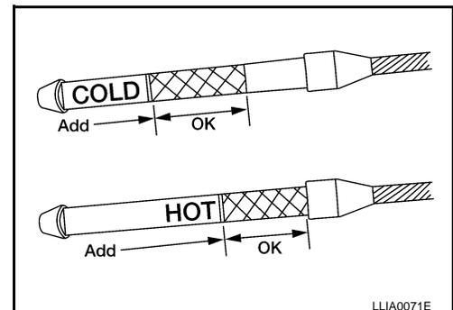
8. Install the A/T fluid level gauge in the charging pipe and install the A/T fluid level gauge bolt.
