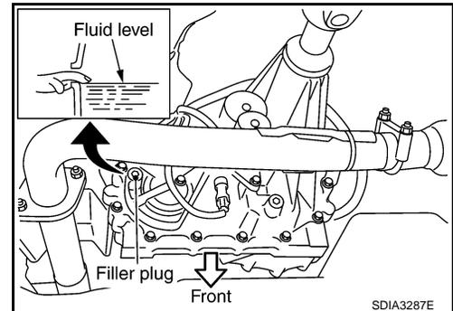
3. Install the filler plug with a new gasket to the transfer. Tighten to the specified torque. Refer to [DLN-149, "Disassembly and Assembly"](#) (ATX14B), [DLN-288, "Disassembly and Assembly"](#) (TX15B).
