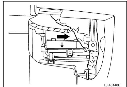
5. Install the in-cabin microfilter cover.
