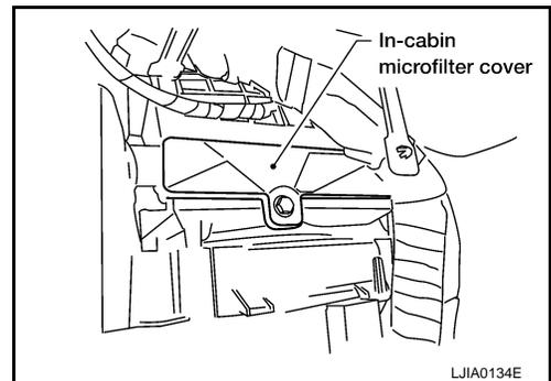
4. Insert the first new in-cabin microfilter into the front heater and cooling unit housing and slide it over to the right. Insert the second new in-cabin microfilter into the front heater and cooling unit housing.
