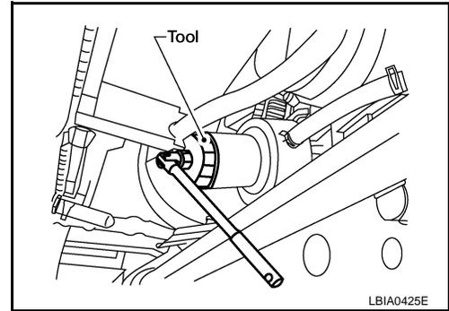
3. Remove any foreign materials adhering to the oil filter installation surface.
