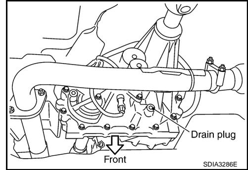
3. Install the drain plug with a new gasket to the transfer. Tighten to the specified torque. Refer to [DLN-149, "Disassembly and Assembly"](#) (ATX14B), [DLN-288, "Disassembly and Assembly"](#) (TX15B).
