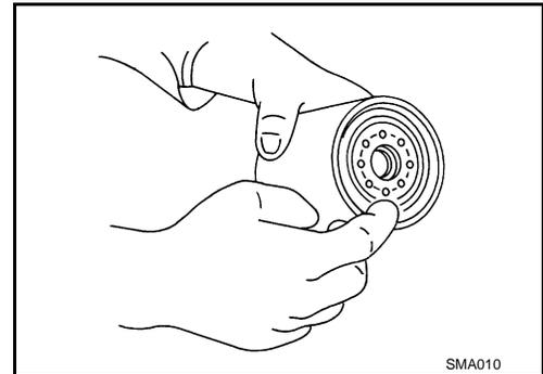
5. Screw on the oil filter manually until a slight resistance is felt, then tighten the oil filter an additional 2/3 turn as shown. Or tighten to specification.
