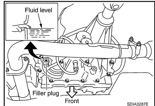
2. Fill the transfer with new fluid until the fluid level reaches the specified limit near the filler plug hole.
