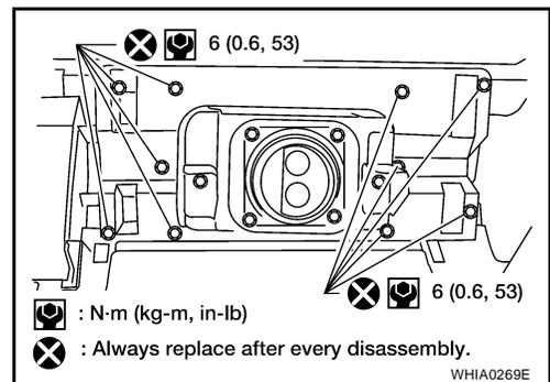
2. Install the instrument panel assembly. Refer to [IP-10, "INSTRUMENT PANEL ASSEMBLY"](#) .
