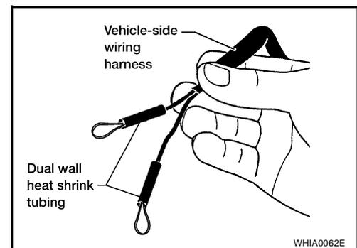
6. Use a heat gun to shrink the heat shrink tubing and seal the wire.
