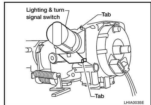
7. Remove the screws. Then while pressing the tab, pull the spiral cable away from steering column assembly.
