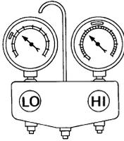
AC356A | High- and low-pressure sides become equal soon after compressor operation stops. | Compressor pressure operation is improper.<br>↓<br>Damaged inside compressor packings. | Replace compressor. |
