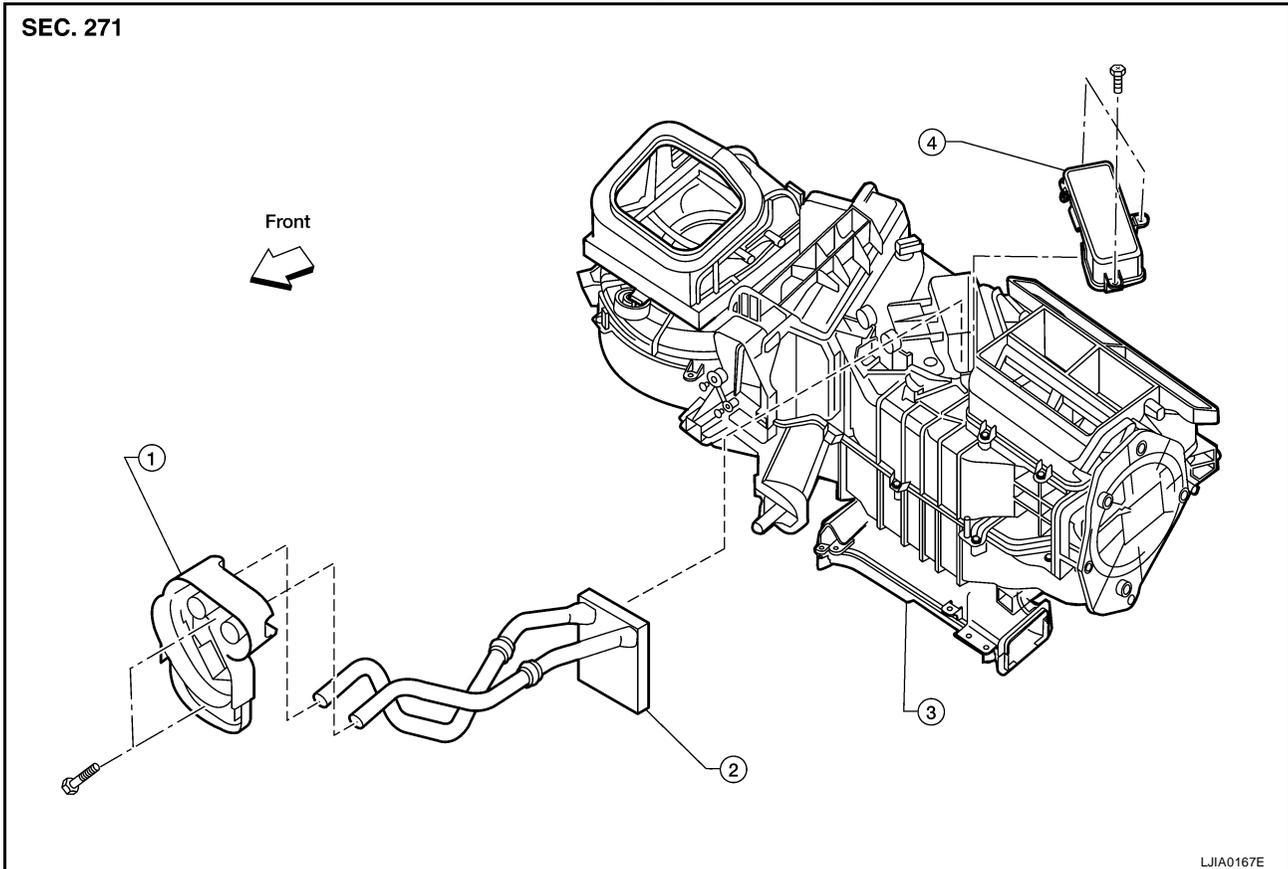
1. Heater core and evaporator pipe bracket 2. Heater core 3. Heater and cooling unit assembly
