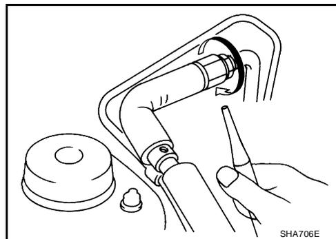
3. Move the probe along each component at a speed of approximately 25 - 50 mm (1 - 2 in)/second as shown.
