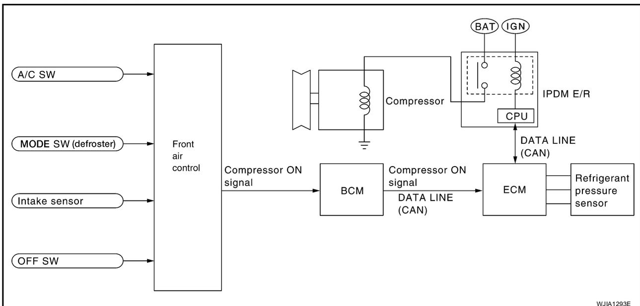
When the A/C switch is pressed, or the mode dial is turned to the defroster position, the front air control outputs a compressor ON signal to BCM.
