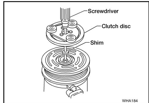
5. Install the clutch pulley bolt using Tool, to prevent the clutch disc from turning and tighten the bolt to specification. Refer to [MTC-102, "COMPONENTS"](#).
