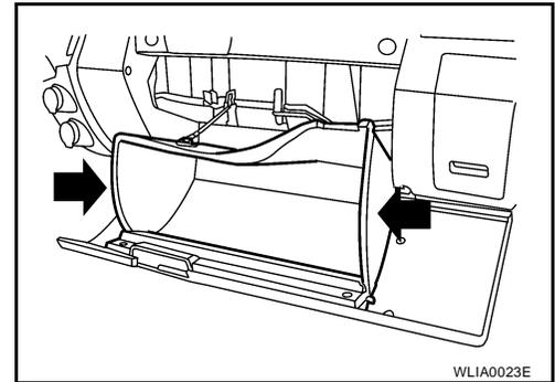
2. Remove the screw and remove the in-cabin microfilter cover.
