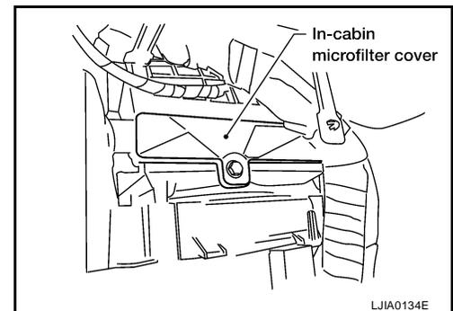
4. Insert the first new in-cabin microfilter into the heater and cooling unit housing and slide it over to the right. Insert the second new in-cabin microfilter into the heater and cooling unit housing.
