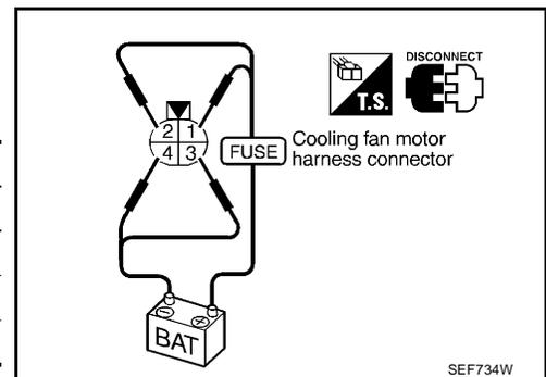
**Cooling fan motor should operate.**
