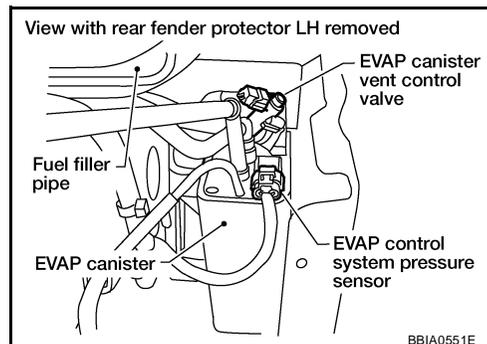
4. Check voltage between EVAP canister vent control valve terminal 1 and ground with CONSULT-II or tester.
