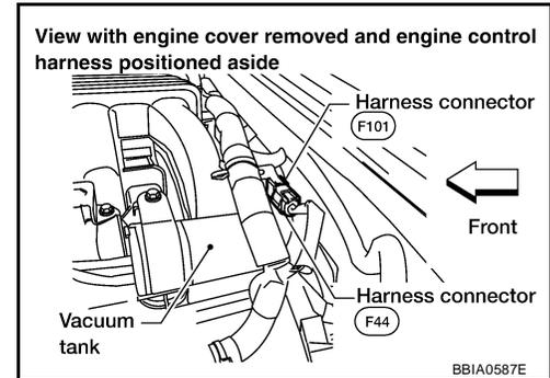
4. Check voltage between harness connector F44 terminal 3 and ground with CONSULT-II or tester.
