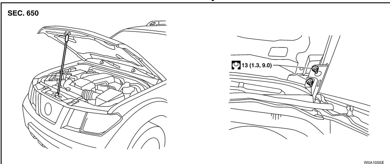
1. Support the hood striker with suitable tool to prevent it from falling.
