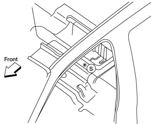
**(T t)** Lower seat belt shoulder height adjuster bolt hole
