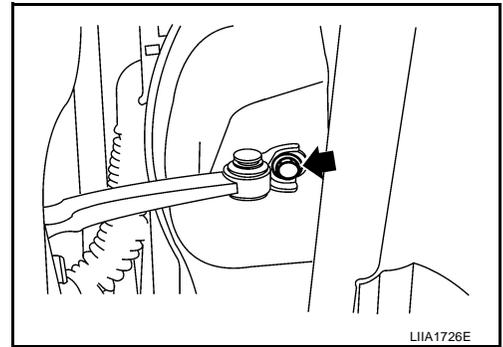
6. Remove the door-side hinge nuts, and remove the door assembly.
