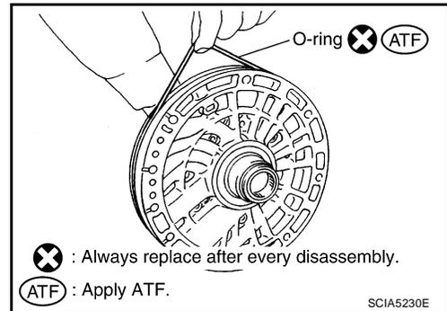
2. Install O-ring to oil pump housing.
