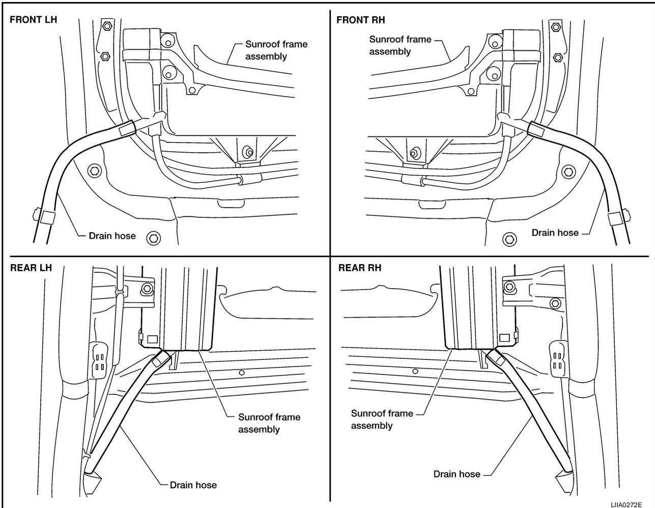
2. Visually check the drain hoses for proper connections, damage or deterioration.
