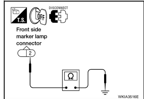
3. Check continuity between front parking lamp harness connector and ground.
