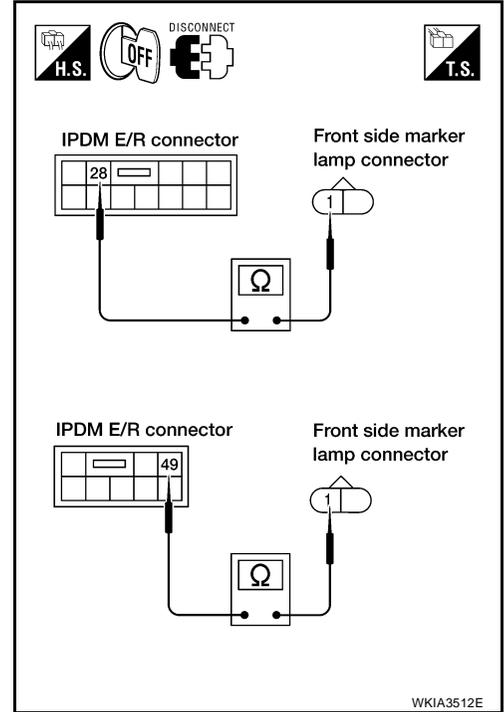
4. Check continuity between IPDM E/R harness connector and front parking lamp harness connector.
