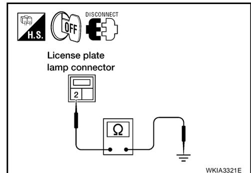
5. Check continuity between rear combination lamp harness connector and ground.
