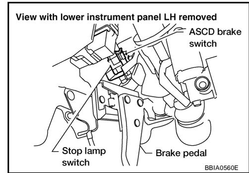
2. Check continuity between stop lamp switch terminals 1 and 2 under the following conditions.
