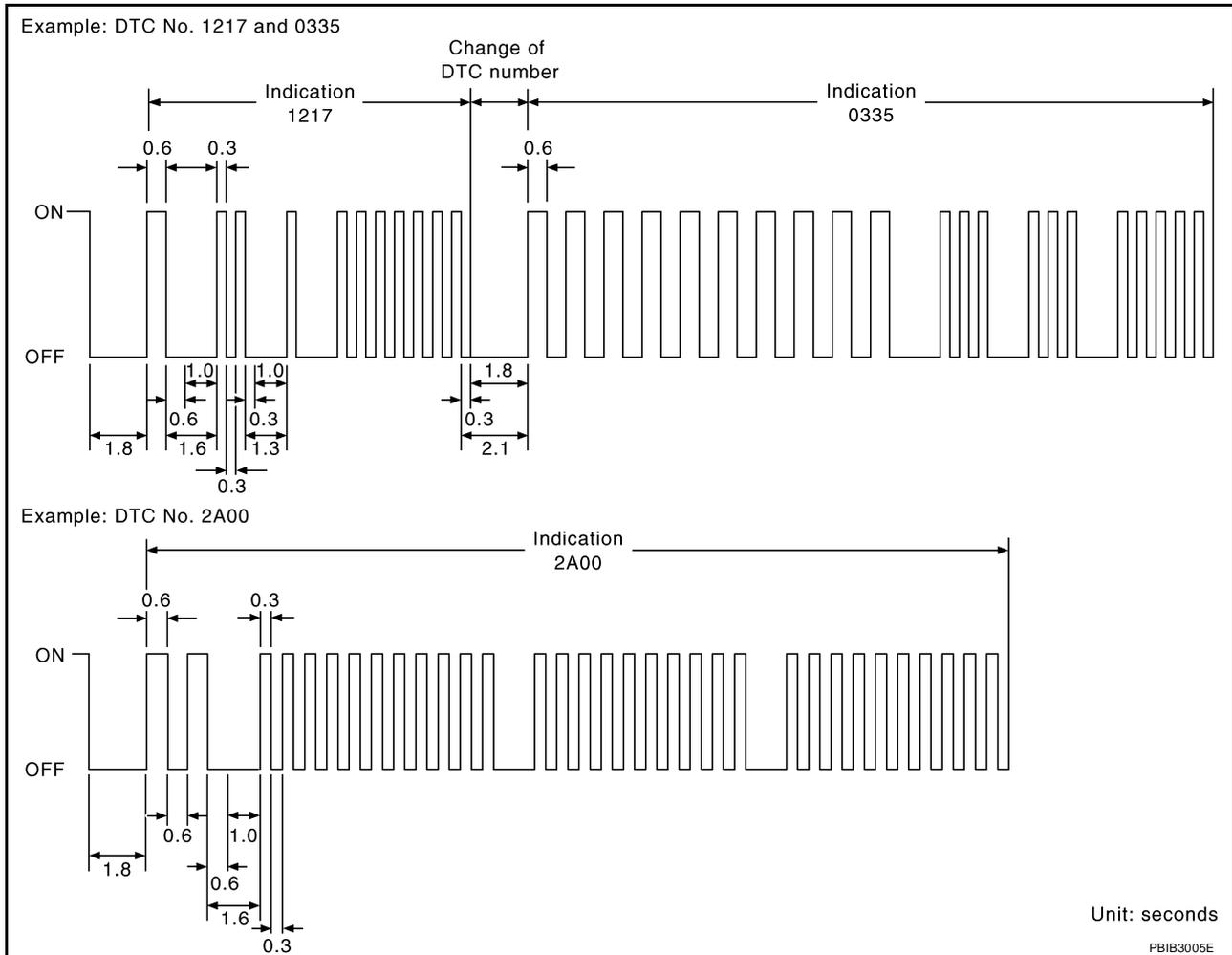
A particular trouble code can be identified by the number of four-digit numeral flashes. The “zero” is indicated by the number of ten flashes. The “A” is indicated by the number of eleven flash. The length of time the 1,000th-digit numeral flashes on and off is 1.2 seconds consisting of an ON (0.6-second) - OFF (0.6-second) cycle.
