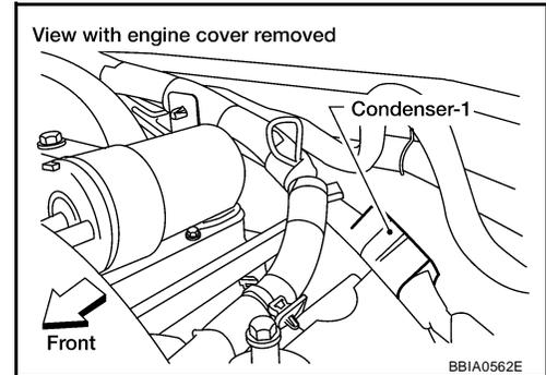
4. Check voltage between condenser-1 terminal 1 and ground with CONSULT-II or tester.
