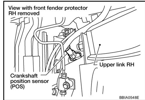
3. Check voltage between CKP sensor (POS) terminal 1 and ground with CONSULT-II or tester.
