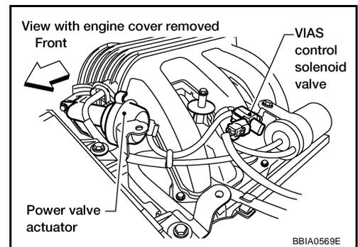
4. Check voltage between terminal 1 and ground with CONSULT-II or tester.
