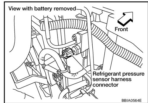
3. Check voltage between refrigerant pressure sensor terminal 3 and ground with CONSULT-II or tester.
