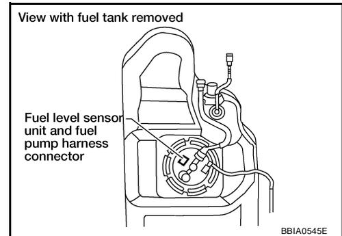
4. Check voltage between "fuel level sensor unit and fuel pump" terminal 4 and ground with CONSULT-II or tester.
