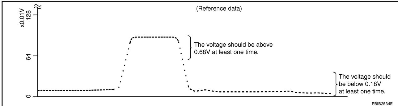
"HO2S2 (B1)/(B2)" should be above 0.68V at least once when the "FUEL INJECTION" is +25%.
