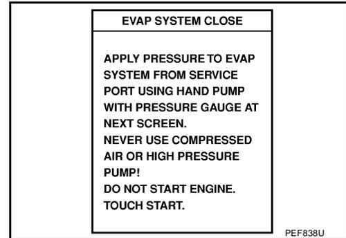
6. Apply positive pressure to the EVAP system until the pressure indicator reaches the middle of the bar graph.
