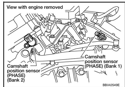
3. Check voltage between CMP sensor (PHASE) terminal 3 and ground with CONSULT-II or tester.
