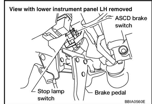
4. Check voltage between ASCD brake switch terminal 1 and ground with CONSULT-II or tester.
