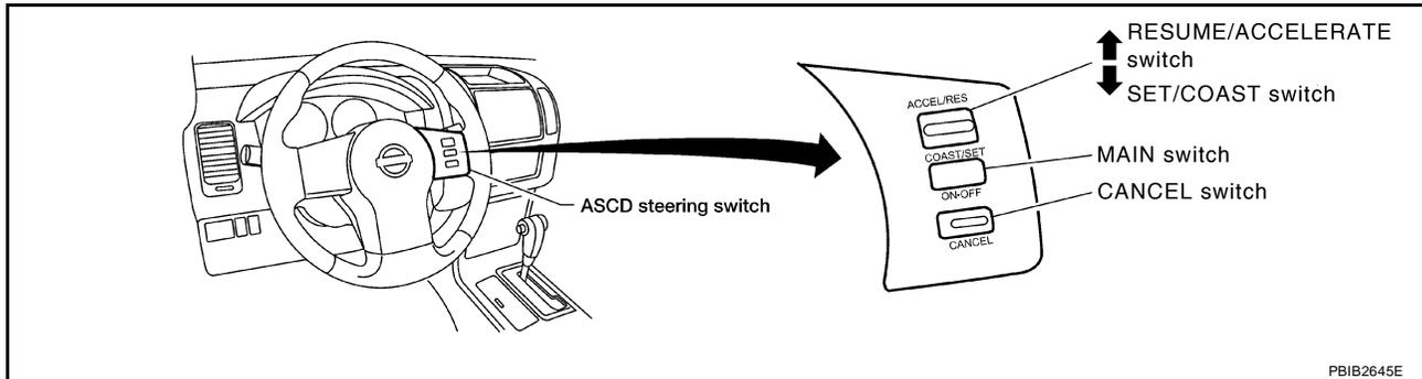
Refer to [EC-29, "AUTOMATIC SPEED CONTROL DEVICE \(ASCD\)"](#) for the ASCD function.
