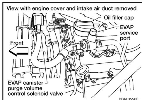
4. Check voltage between EVAP canister purge volume control solenoid valve terminal 2 and ground with CONSULT-II or tester.
