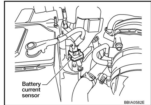
3. Check voltage between battery current sensor terminal 1 and ground with CONSULT-II or tester.
