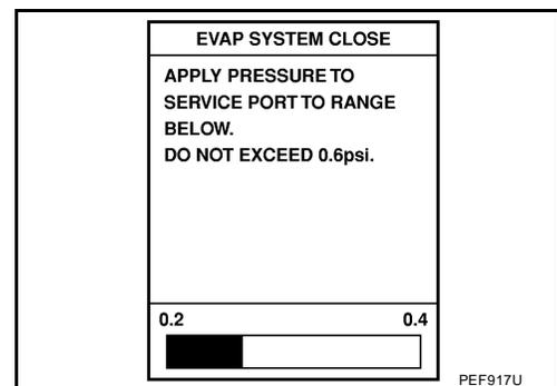
8. Locate the leak using a leak detector. Refer to [EC-33, "EVAPORATIVE EMISSION LINE DRAWING"](#).
