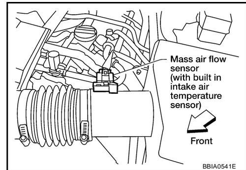
3. Check voltage between mass air flow sensor terminal 5 and ground.
