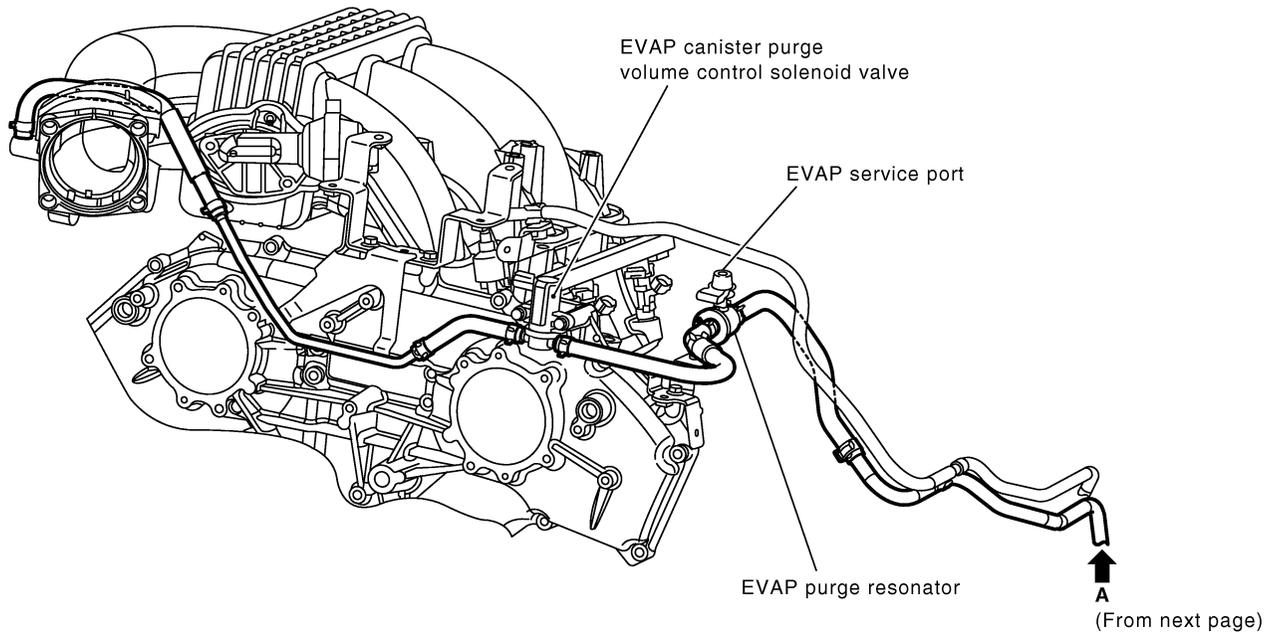
**NOTE: Do not use soapy water or any type of solvent while installing vacuum hose or purge hoses.**
