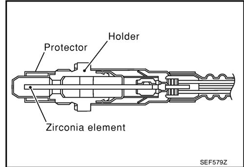
An electronic circuit controls the pump current through the oxygen-pump cell so that the composition of the exhaust gas in the diffusion gap remains constant at  $\lambda = 1$ . Therefore, the A/F sensor is able to indicate air/fuel ratio by this pumping of current. In addition, a heater is integrated in the sensor to ensure the required operating temperature of 700 - 800°C (1,292 - 1,472°F).
