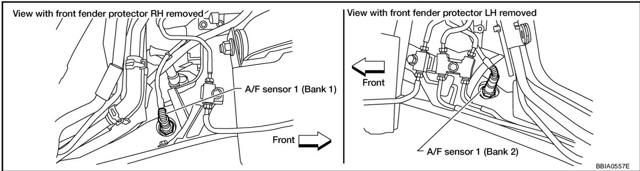
**Tightening torque: 50 N-m (5.1 kg-m, 37 ft-lb)**
