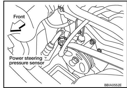
3. Check voltage between PSP sensor terminal 3 and ground with CONSULT-II or tester.
