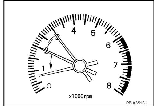
3. Read idle speed in "DATA MONITOR" mode with CONSULT-II. Refer to [EC-75, "IDLE SPEED"](#) .
