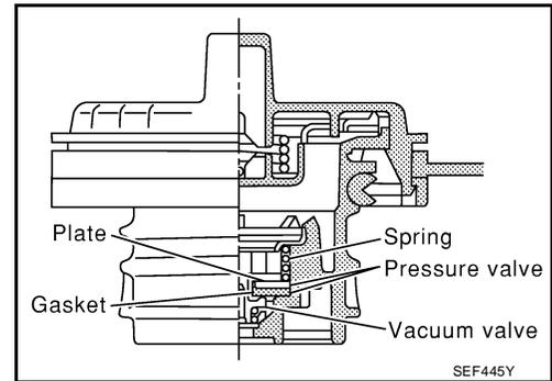
2. Check valve opening pressure and vacuum.
