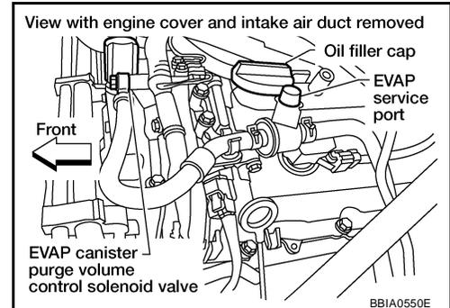
4. Check voltage between EVAP canister purge volume control solenoid valve terminal 2 and ground with CONSULT-II or tester.
