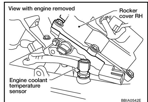
3. Check voltage between ECT sensor terminal 1 and ground with CONSULT-II or tester.
