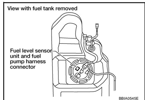
5. Check voltage between "fuel level sensor unit and fuel pump" terminal 1 and ground with CONSULT-II or tester.
