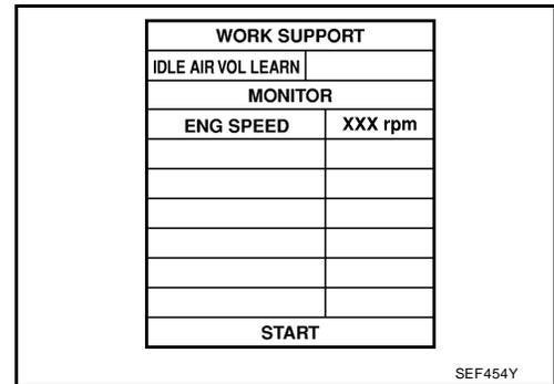
7. Make sure that "CMPLT" is displayed on CONSULT-II screen. If "CMPLT" is not displayed, Idle Air Volume Learning will not be carried out successfully. In this case, find the cause of the incident by referring to the Diagnostic Procedure below.
