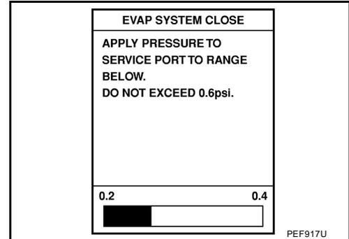
4. Using EVAP leak detector, locate the EVAP leak. For the leak detector, refer to the instruction manual for more details. Refer to [EC-33, "EVAPORATIVE EMISSION LINE DRAWING"](#).
