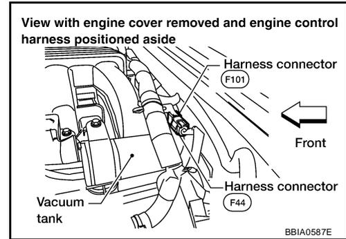
4. Check voltage between harness connector F44 terminal 3 and ground with CONSULT-II or tester.
