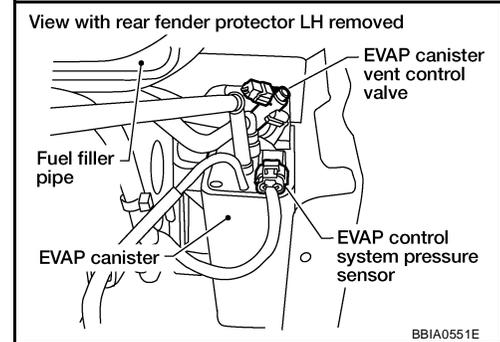
4. Check voltage between EVAP canister vent control valve terminal 1 and ground with CONSULT-II or tester.
