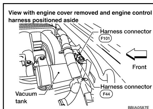
3. Check voltage between harness connector F44 terminal 3 and ground with CONSULT-II or tester.
