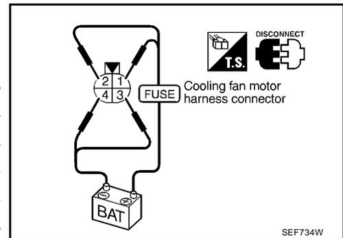
**Cooling fan motor should operate.**
