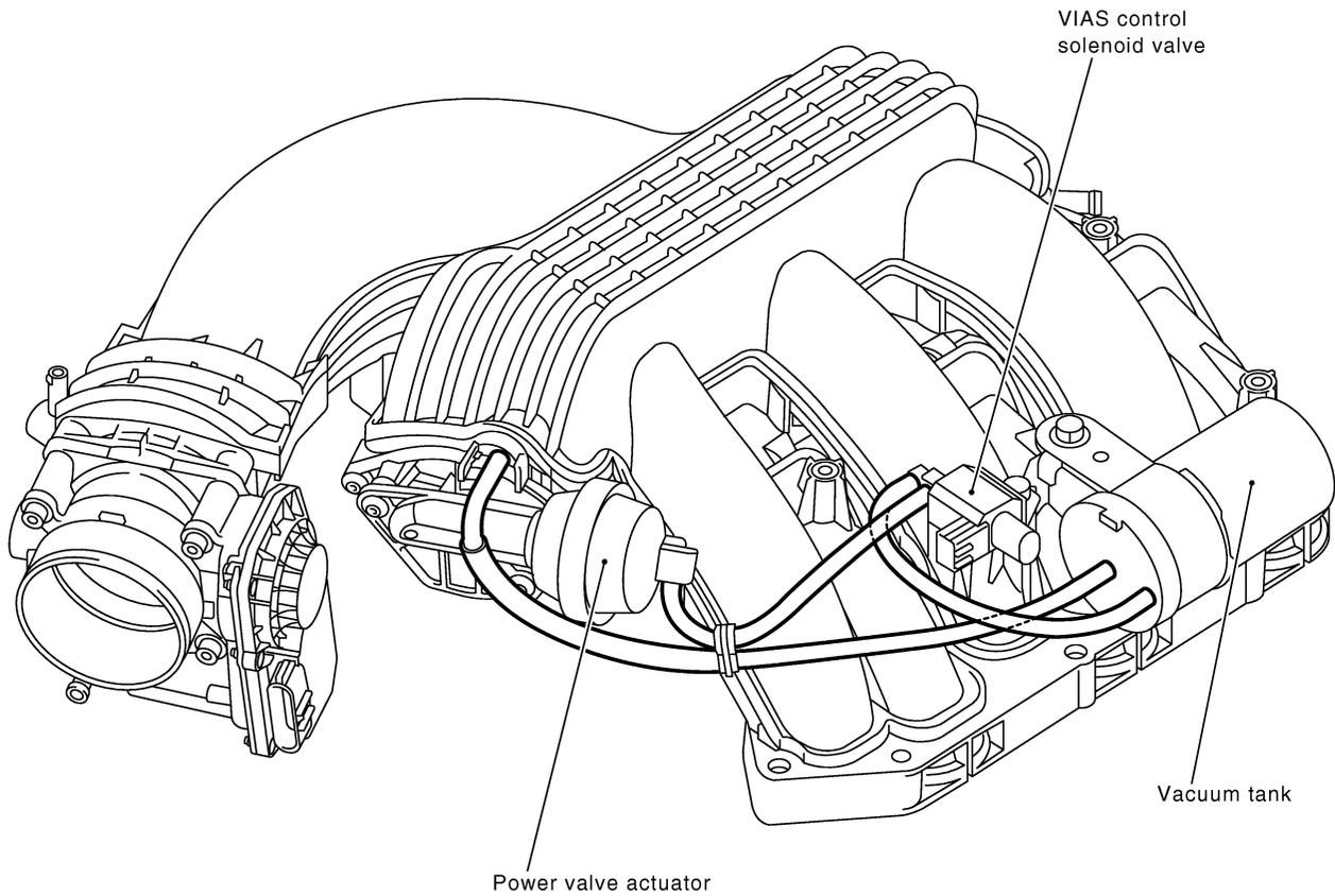
**NOTE:** Do not use soapy water or any type of solvent while installing vacuum hose or purge hoses.
