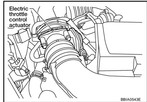
3. Check voltage between electric throttle control actuator terminal 2 and ground with CONSULT-II or tester.
