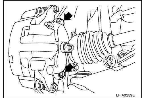
5. Install brake hose to cylinder body, if removed, then tighten union bolt to the specified torque. Refer to [BR-24, "Components"](#) .
