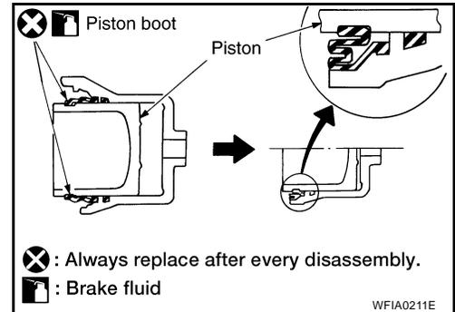
4. Insert into cylinder body by hand and insert piston boot piston-side lip into piston groove.
