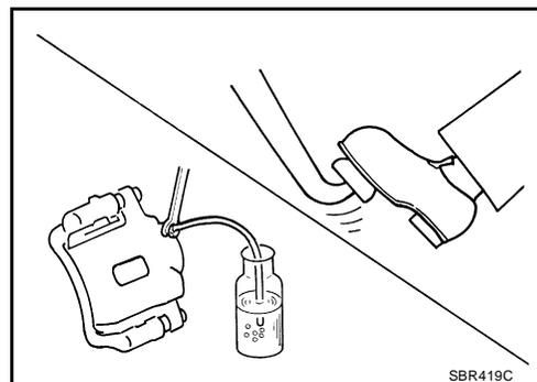
3. Make sure there is no foreign material in reservoir tank, and refill with new brake fluid.
