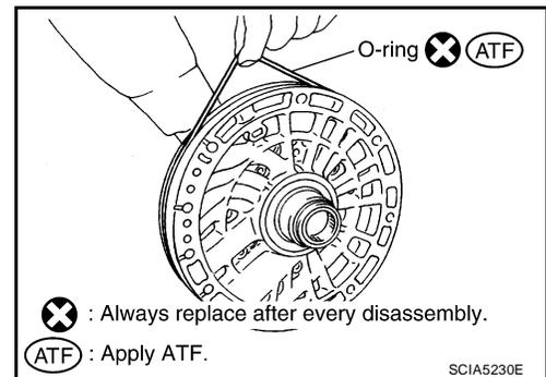
2. Install O-ring to oil pump housing.
