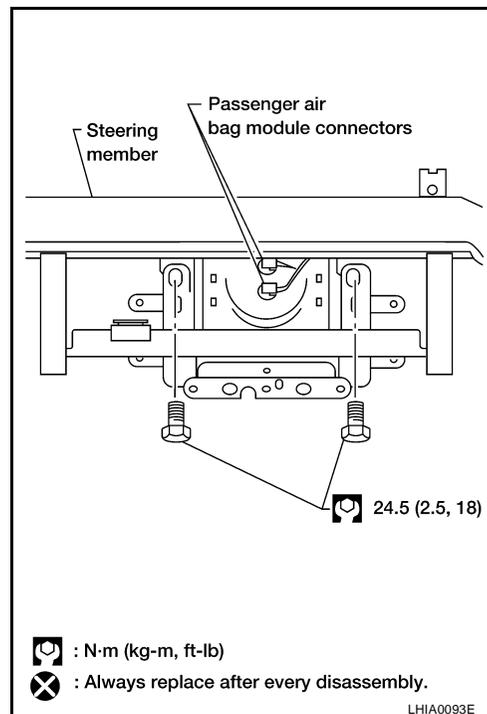
5. Remove front passenger air bag module screws then remove passenger air bag module from instrument panel assembly.
