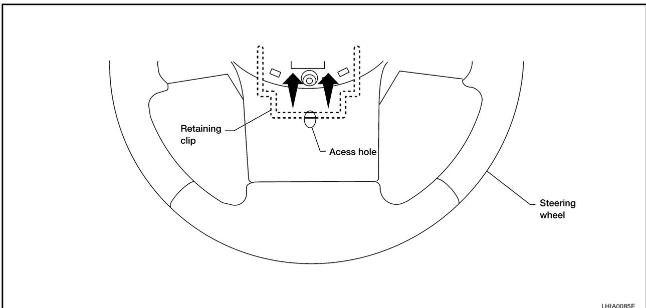
2. Press upward (toward center of steering wheel) on retaining clip until driver air bag module is released from steering wheel.
