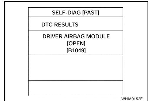
If no malfunction is detected on "SELF-DIAG [PAST]", touch "BACK" and go back to "SELECT DIAG MODE".
