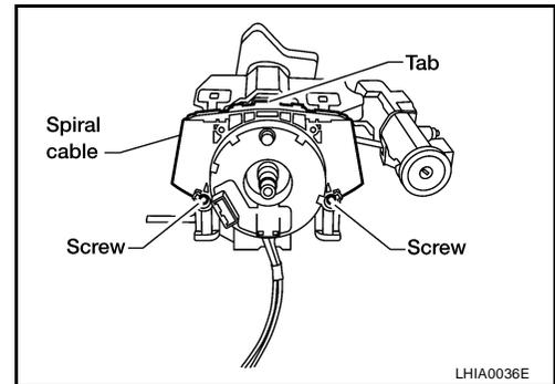
7. Disconnect the spiral cable connectors.
